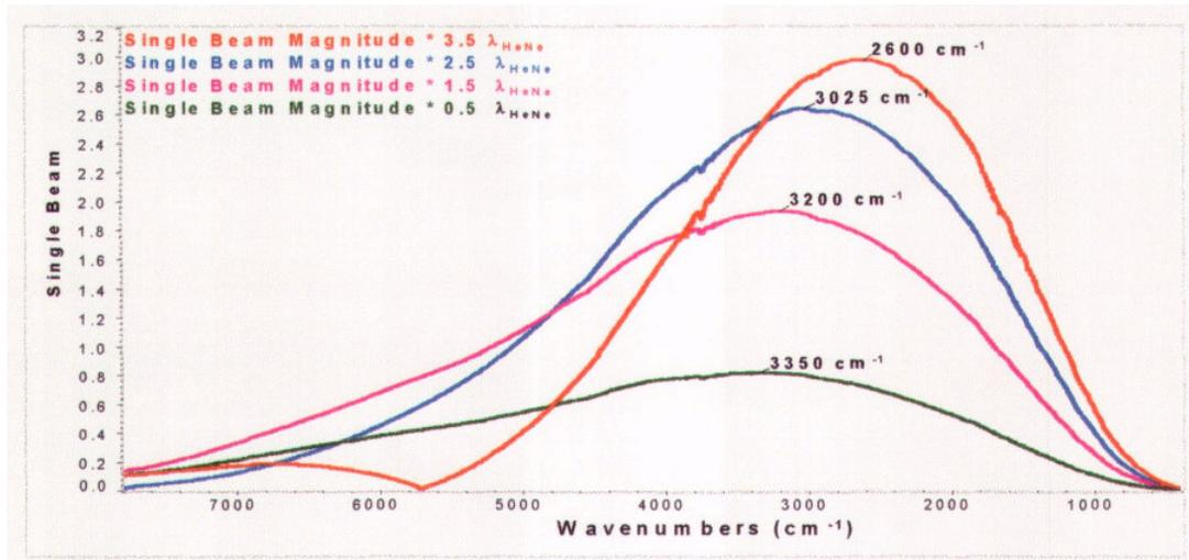
The PM amplitude should be chosen according to the spectral range of interest. PM amplitudes of  $0.5 \lambda_{\text{HeNe}}$  or  $1.5 \lambda_{\text{HeNe}}$  are appropriate for a near infrared experiment. The PM amplitude of  $3.5 \lambda_{\text{HeNe}}$  provides an excellent coverage over the entire mid-IR region. Larger PM amplitudes will shift the largest lobe to lower energies and, at the same time, will bring nodes into mid-IR region.
