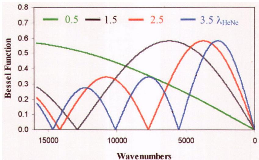
All Bessel functions share the following characteristics: (1) *The first lobe (from low energy) is the largest and the ones at higher energies become increasingly smaller in magnitude.* (2) *The lobes become narrower and shift to lower energies as the PM amplitude increases.*
