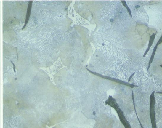
29.1 In reflected-light brightfield, the fine structures in the iron casting are difficult to see.
