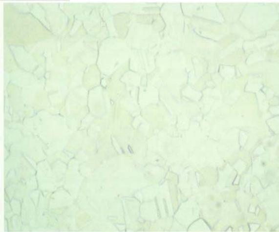
The structure of this brass sample can be seen only very faintly in reflected-light brightfield.
