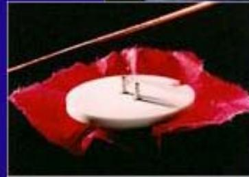
W Filament - Current density  $\sim 10\text{A}/\text{cm}^2$ , probe size  $\sim 5.0\text{nm}$
