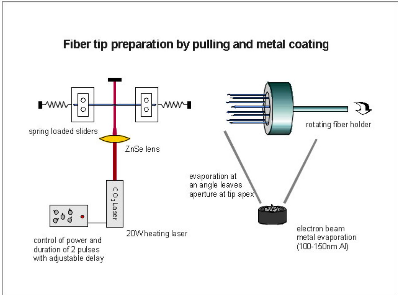
The most crucial part of a near-field optical microscope is the **optical probe**. In most cases it is fabricated from an optical fiber which has been tapered (to reduce its size) and coated with metal
