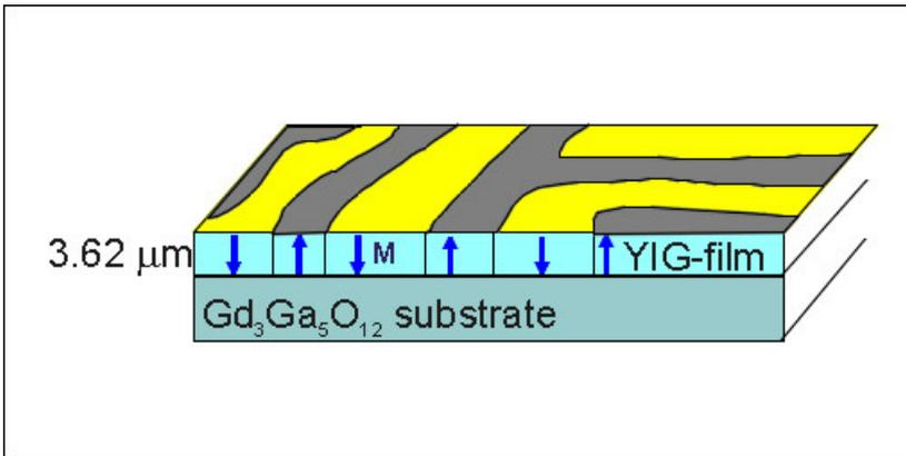
Bismuth-doped yttrium-iron-garnet film (YIG) films exhibit perpendicular magnetization, their domains can be imaged by applying the polarization modulation scheme. In contrast to the experiments on the dye crystals described above, this sample displays no polarization-dependent absorption, and an
