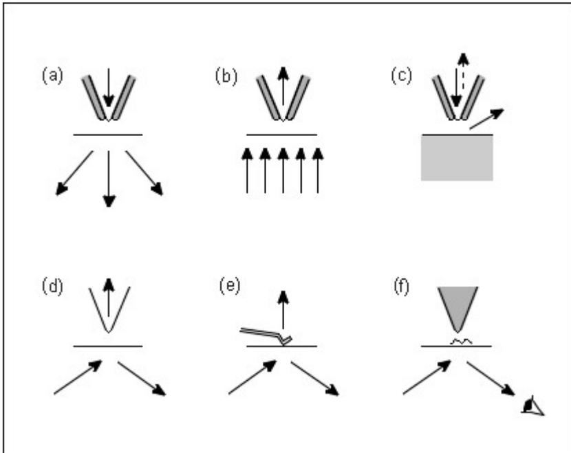
tip on a cantilever (e). In the Plasmon Near-Field microscope, surface plasmons are generated at the surface of a sample on a thin film metallic substrate, and scattered by a probe tip (f).
