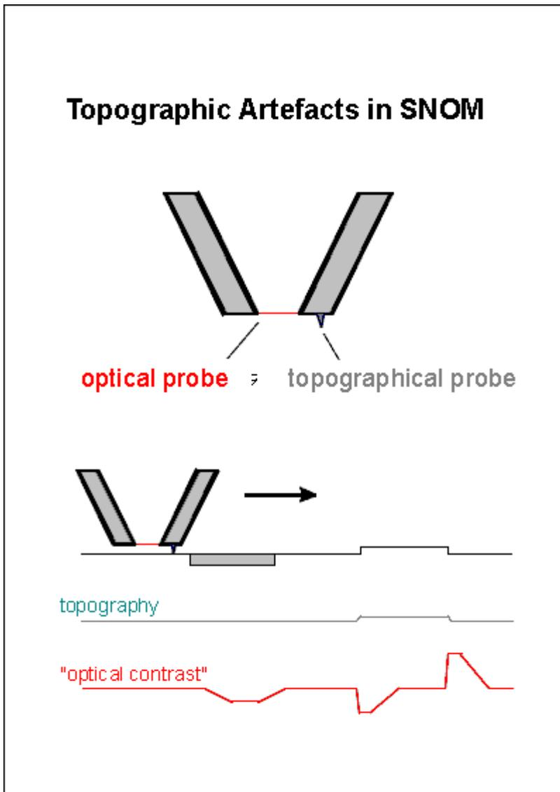
Care has to be taken when SNOM images are acquired while the fiber probe follows the surface topography. The near-field optical signal is strongly dependent on the distance of the optical probe to the sample surface. Therefore, only slight changes of this distance are already enough to considerably change the recorded optical signal. So far, so good.
