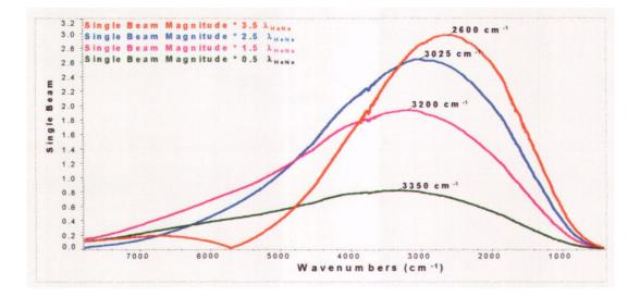
The PM amplitude should be chosen according to the spectral range of interest. PM amplitudes of  $0.5 \lambda_{HeNe}$  or  $1.5 \lambda_{HeNe}$  are appropriate for a near infrared experiment. The PM amplitude of  $3.5 \lambda_{HeNe}$  provides an excellent coverage over the entire mid-IR region. Larger PM amplitudes will shift the largest lobe to lower energies and, at the same time, will bring nodes into mid-IR region.
