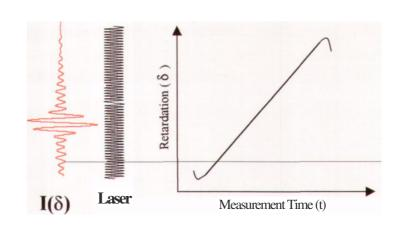
measured at precisely equal intervals of mirror positions and provides an internal wavelength calibration for every scan *(Cannes Advantage)*. \*
