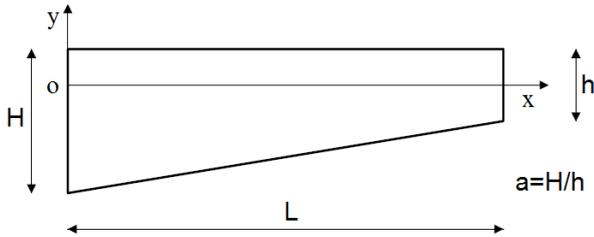
Figure 2: Non-symmetric tapered beam geometry
