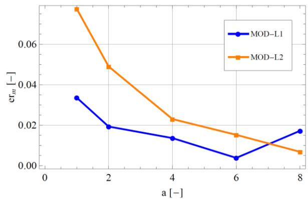
**Figure 6:** Symmetric tapered beam, Stiffness matrix average error varying the taper ratio  $a=H/h$  and length  $L$ , for 2D model for  $H/L_1=1/10$  and  $H/L_2=1/5$  (respectively MOD-L1 and MOD-L2).
