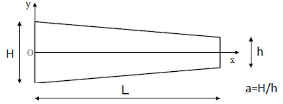
**Figure 3:** Symmetric tapered beam geometry
