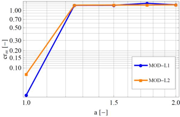
**Figure 5:** Non-symmetric tapered beam, Stiffness matrix average error varying the taper ratio  $a=H/h$  from 1 to 2 and length  $L$ , for 2D model for  $H/L_1=1/10$  and  $H/L_2=1/5$  (respectively MOD-L1 and MOD-L2).
