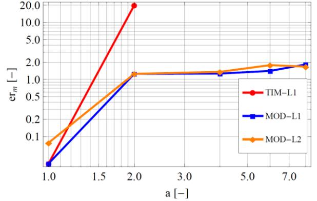
**Figure 4:** Non-symmetric tapered beam, Stiffness matrix average error varying the taper ratio  $a=H/h$  from 1 to 8, for Timoshenko theory (TIM) and 2D model for  $H/L1=1/10$  and  $H/L2=1/5$  (respectively MOD-L1 and MOD-L2).
