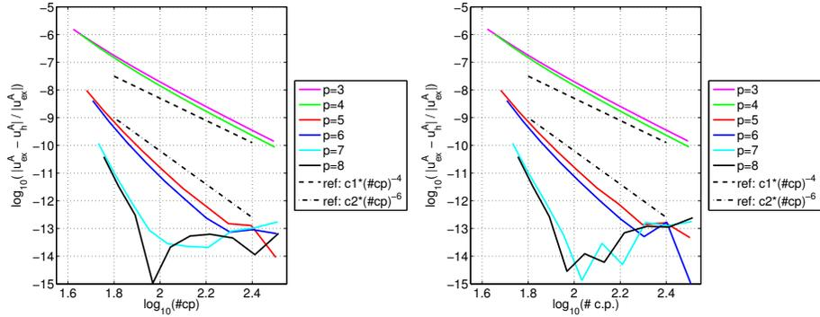
FIGURE 4. Circular arch with out-of-plane load, solved by a mixed collocation method with  $p_v = p_\varphi - 1 = p_n - 2 = p$ .  $L^2$ -norm of displacements error versus number of total collocation points, for  $t/r = 10^{-1}$  (left) and  $t/r = 10^{-4}$  (right). Dashed lines indicate reference orders of convergence.
