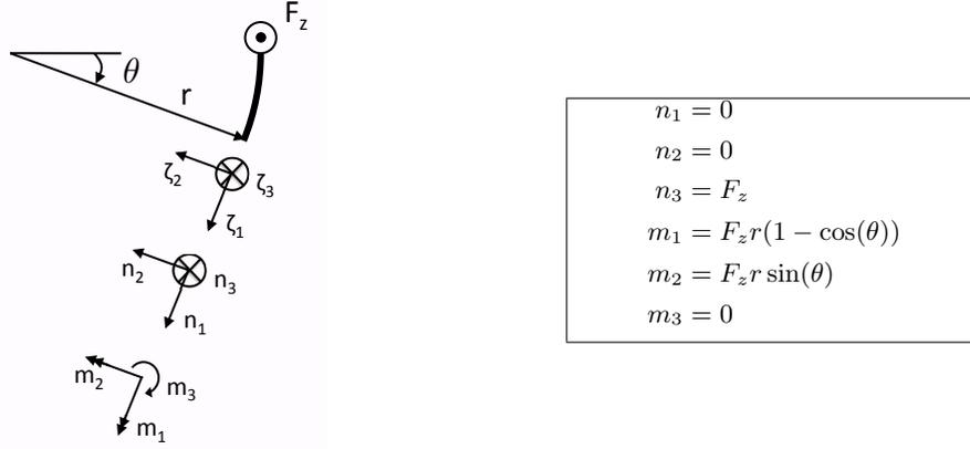
FIGURE 2. Stress resultant functions for the circular arch.
