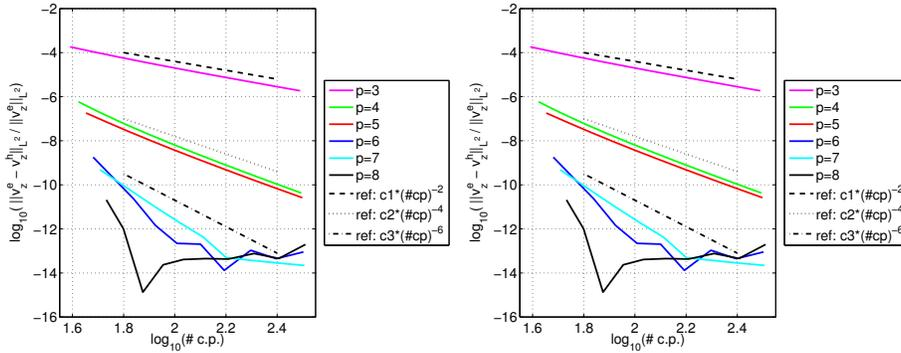
FIGURE 3. Circular arch with out-of-plane load, solved by a mixed collocation method with  $p_v = p_\varphi = p_n = p$ .  $L^2$ -norm of displacements error versus number of total collocation points, for  $t/r = 10^{-1}$  (left) and  $t/r = 10^{-4}$  (right). Dashed lines indicate reference orders of convergence.
