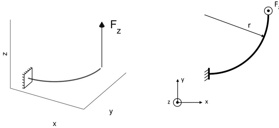
FIGURE 1. Circular arch with out-of-plane load. Perspective view (a) and top view (b).
