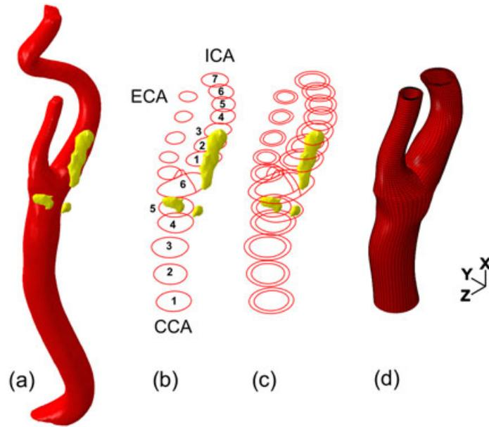
Figure 2. Generation of carotid artery wall mesh: (a) 3D reconstruction of vessel lumen and plaque; (b) closed lines representing the inner cross-sectional profile; (c) closed lines representing the inner and outer cross-sectional profiles; and (d) carotid artery wall mesh.
