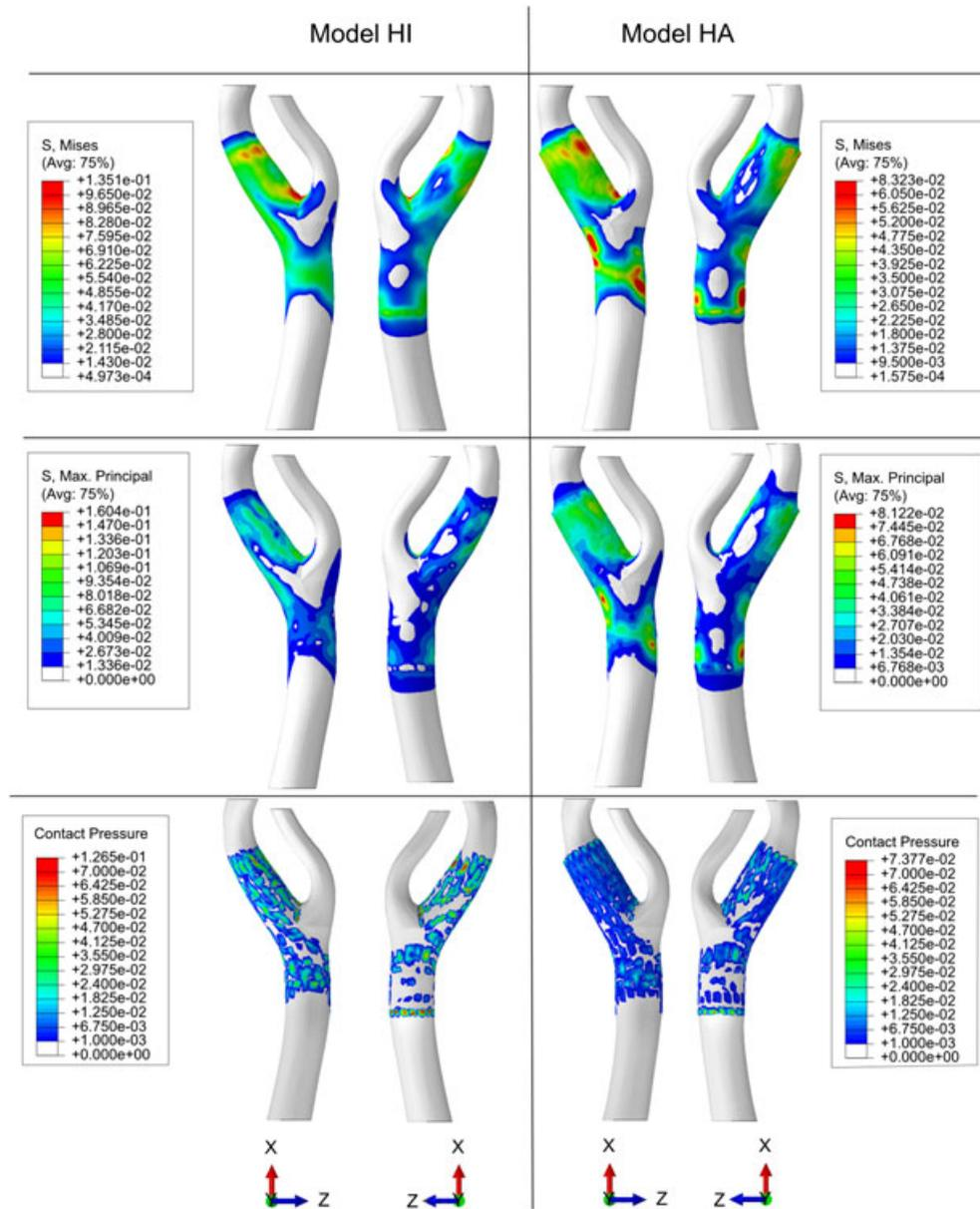
Figure 8. Post-stenting  $\sigma_M$  (top), maximum principal stress (middle) and contact pressure (bottom) distribution over the inner vessel wall (front and back views). With respect to  $\sigma_M$ , the color bar is rescaled by setting the corresponding  $\sigma_M^{99P}$  as the maximum and  $\sigma_M^{Mean}$  as the minimum. MPa is the unit of measure.
