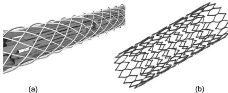
Figure 6. a) three-dimensional reconstruction of an 8.45-mm portion of the stent (dark gray) within the delivery sheath (light gray); b) finite element model of the open-cell stent in free expanded configuration.
