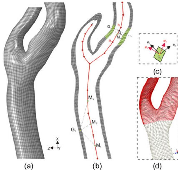
Figure A.1. (a) Mesh of the carotid artery model; (b) example of local coordinate system definition; (c) local cylindrical coordinate system rotation to accomplish element orientation; and (d) obtained collagen fiber distribution (circumferential and axial direction) at bifurcation for common carotid artery (white) and internal carotid artery/external carotid artery (red).
