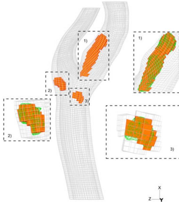
Figure 4. Inclusion of the plaque in the carotid artery vessel model: the plaque (orange) is defined assessing the elements of the vessel wall mesh (gray) enclosed within 3D stereolithography surface (green) representing the plaque morphology.
