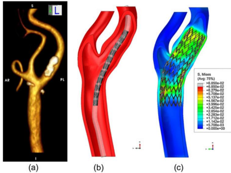
Figure 7. Finite element analysis of carotid artery stenting: (a) 3D reconstruction of carotid artery lumen from computed tomography angiography images; (b) stent crimped in the delivery system during the simulation; (c) contour plot depicting the post-stenting stress distribution over the vessel wall (model  $HA$ ) at the end of the simulation; the cut-view option is used for the vessel and MPa is the unit of measure for  $\sigma_M$ .
