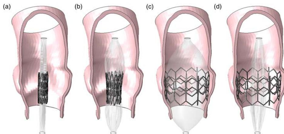
Figure 5. Different frames of balloon expansion and stent apposition: (a) initial configuration; (b) the balloon starts to deploy the stent; (c) the balloon is fully expanded and the stent fully deployed; (d) final configuration after balloon deflation.
