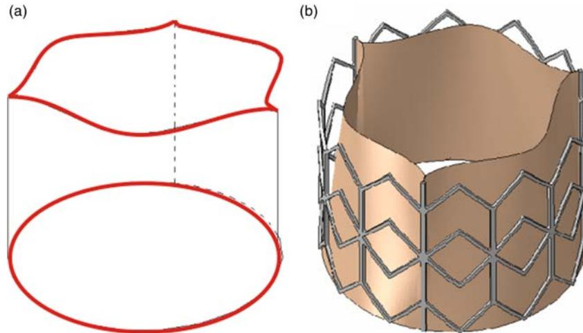
Figure 6. The Edwards SAPIEN model: (a) the valve is created by means of a lofting procedure carried out between the bottom and top curve highlighted in red; (b) the whole device model made of the stent and the valve is shown.
