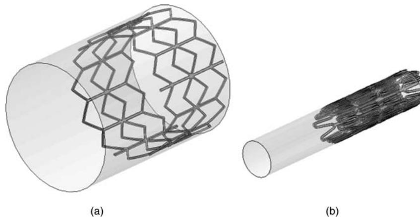
Figure 2. Simulation of stent crimping: (a) at the beginning a rigid catheter is created around the undeformed geometry of the stent; (b) the catheter is gradually crimped leading to stent deformation.
