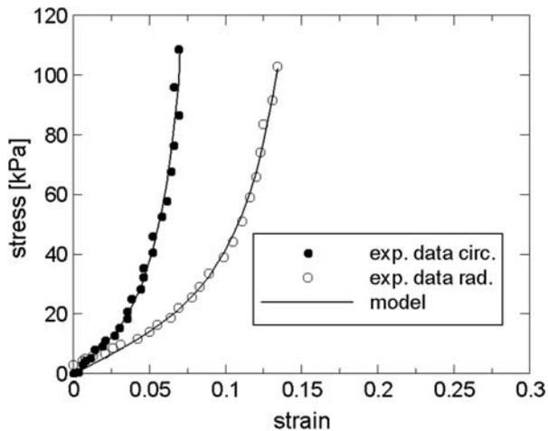
Figure 4. Experimental data versus model prediction: circumferential and radial stress–strain responses of human aortic sinuses (Martin et al. 2011) are compared with results obtained with the model by Holzapfel et al. (2000).
