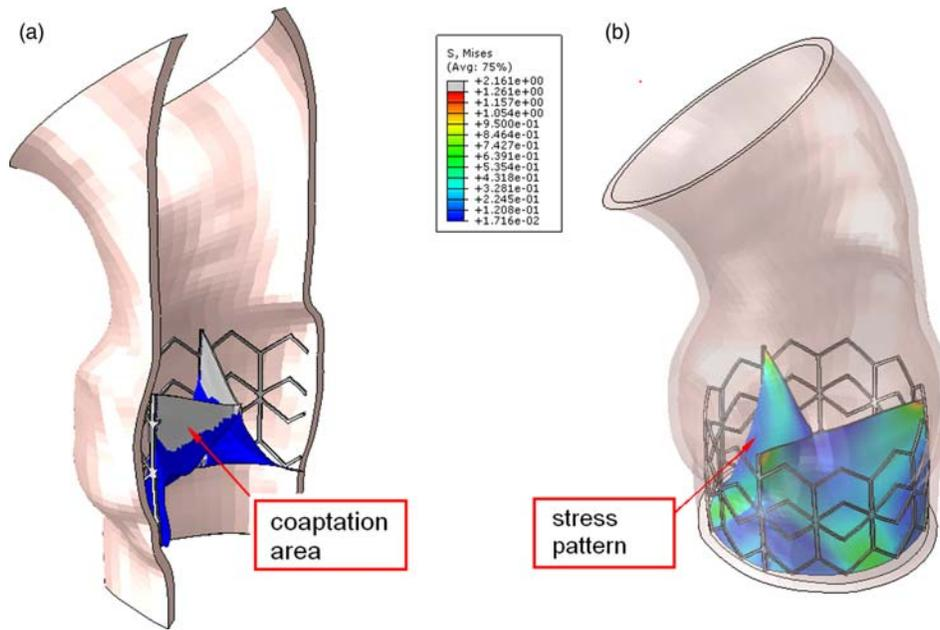
Figure 9. Simulation results: (a) the coaptation area is highlighted; (b) the leaflet tensile state (MPa) is reported.
