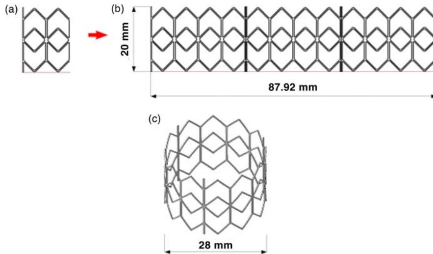
Figure 1. Creation of stent model: (a) a primitive geometry is mirrored and replicated to obtain the model; (b) whole planar model: the stent circumference and height are reported; (c) the nodes of the planar configuration are then expressed in terms of polar coordinates to get the characteristic circular shape: the inner diameter is indicated.
