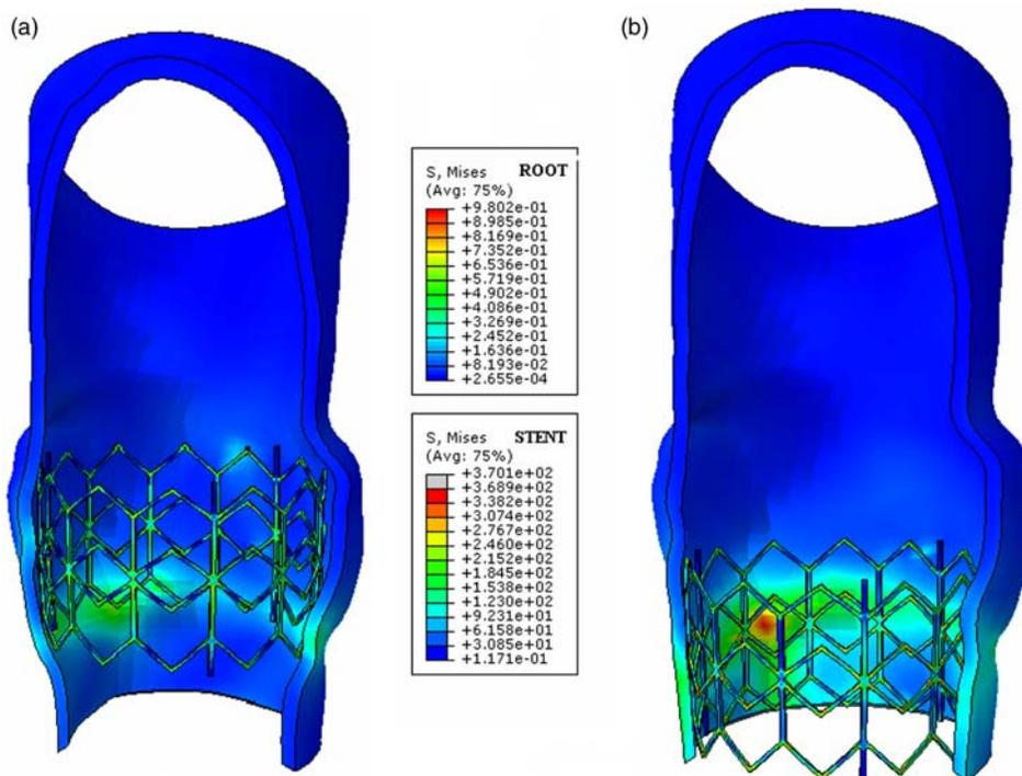
Figure 10. Simulation results: the von Mises stresses on the aortic root wall and stent struts are represented (a) after the distal positioning and (b) after the proximal positioning.
