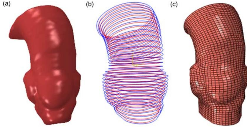
Figure 3. Creation of aortic root model: (a) an STL file is extracted by processing the DICOM images; (b) the inner (red) and outer (blue) lines identifying the aortic root wall are defined from the STL file; (c) a hexahedral element mesh is then created.
