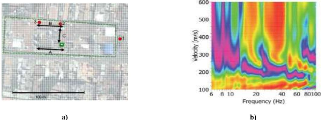
**Fig. 3** Parthasarathy temple (India): a) georeferenced feature map of the temple (green dotted lines), building analyzed with structural tests (green bold lines), seismic lines (black arrows, letters A to C) and Nakamura test locations (red dots, letters 1-3); b) MASW spectra showing phase velocity versus frequency for line A.
