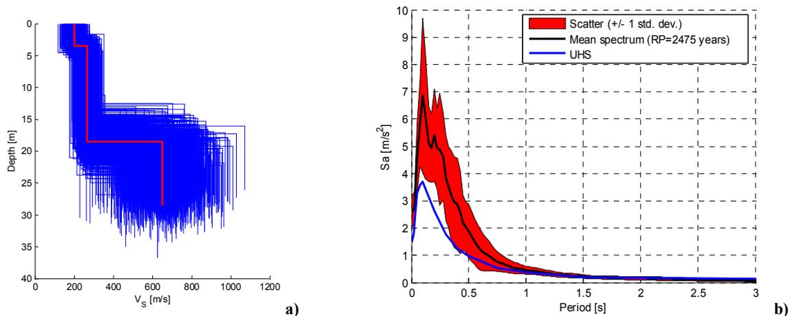
**Fig. 5** Stochastic ground response analyses at the Indian site: a) random profiles obtained using the Latin hypercube sampling technique (the red line represents the mean profile) and b) mean spectrum (black line) plus/minus one standard deviation (red area) at the surface and the UHS obtained from the PSHA (blue line).
