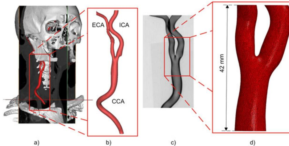
Figure 1. Elaboration of computed tomography angiography images: (a) whole 3D reconstruction of neck-head district highlighting the region of interest; (b) surface describing the carotid artery lumen used to create the silicon artery; (c) radiography of the silicon artery highlighting the non-uniform wall thickness; (d) tetrahedral mesh adopted in the simulations.
