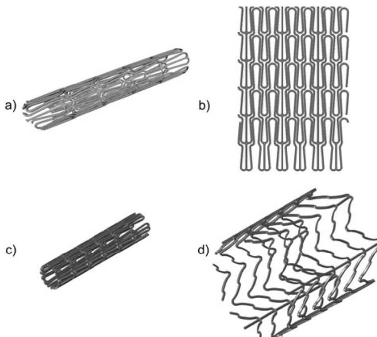
Figure 2. Stent mesh generation: (a) detail of a high resolution micro-CT performed on a real stent within the delivery system; (b) planar CAD geometry resembling the stent design pattern; (c) stent mesh in crimped configuration; (d) stent mesh in free-expanded configuration.
