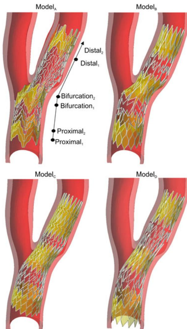
Figure 5. Considered stent designs after the deployment simulation. The cells considered for area computation are depicted in yellow.
