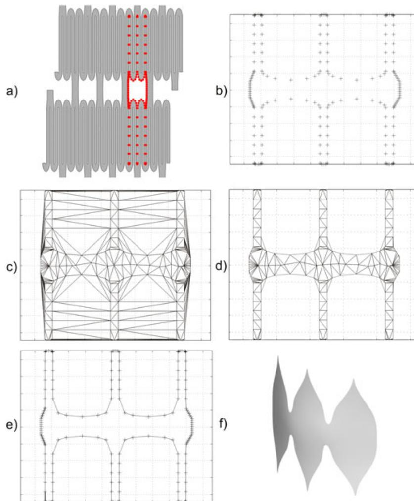
Figure 4. Cell surface definition: (a) and (b) Node identification of cell boundary nodes; (c) Delaunay triangulation of each node set; (d) Delaunay triangulation after the application of distortion criterion; (e) detection of outer edges; (f) and creation of 3D cell surface.
