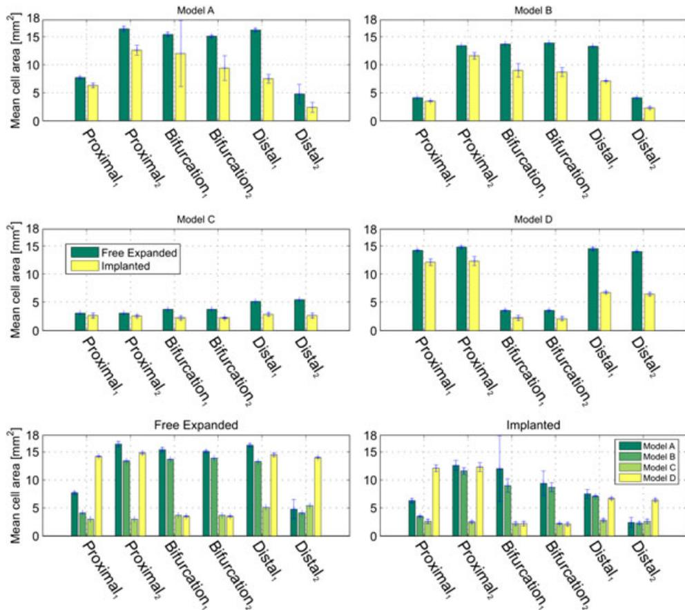
Figure 6. Bar graph of the mean cell area: free expanded versus implanted for each stent model (top and middle); comparison between the stent models in free-expanded configuration (bottom-left) and implanted (bottom-right).
