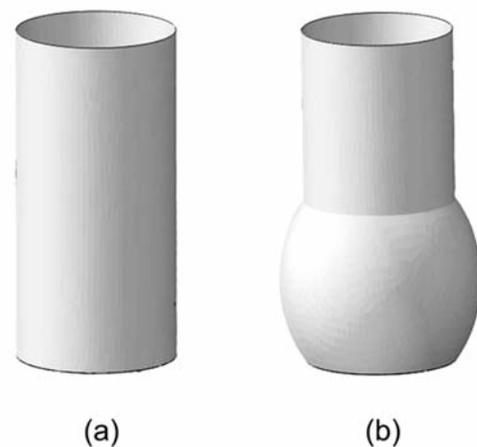
Figure 2: The geometric models of the Dacron grafts adopted for simulation of the AVS procedure. a) The Standard Dacron graft. b) The Valsalva graft.
