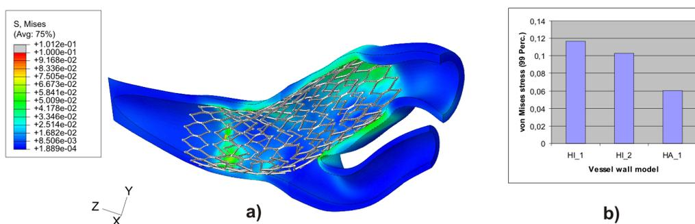
Figure 2: a) contour plot of the von Mises stress distribution in the CA wall after the stent apposition, the results refer to model  $HA_1$ ; b) histograms depicting the maximum von Mises stress value (99 Perc.) as function of the vessel constitutive model. For both figures, MPa is the stress unit measure.
