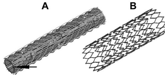
**Figure 3** ♦ (A) 3D reconstruction of an 8.45-mm segment of the stent (arrow) within the catheter. (B) Finite element model of an open-cell stent after the shape-setting simulation.
