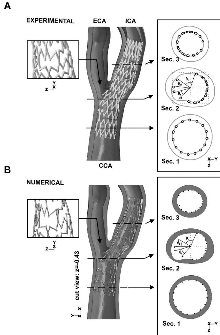
**Figure 6** ♦ Comparison between experimental (A) and numerical (B) stent/vessel configurations. The figure highlights the strut position at 3 sections (1:  $x=10$  mm, 2:  $x=19$  mm, 3:  $x=30$  mm) and the deformation of stent cells from a virtual view through the external carotid artery (ECA). The apparent mismatch of the stent strut thickness between the experimental and numerical results is due only to blooming artifacts in the micro-CT images.
