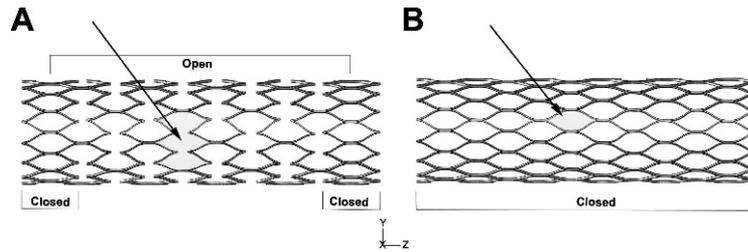
**Figure 5** ♦ Details about the cell arrangement for the (A) open- and (B) closed-cell designs (the standard free cell area is indicated by arrows).
