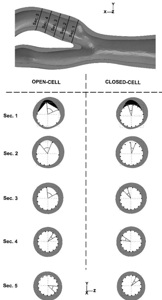
**Figure 8** ♦ Cut views of 5 different vessel cross sections for both open-cell (left) and closed-cell designs (right). The section position is illustrated with respect to the pre-stenting vessel (top); the maximum inter-strut angle for each section is depicted. The gap between the stent and the vessel wall is in black.
