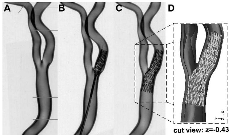
**Figure 4** ♦ (A) Silicone artery: red lines indicate the location of restraints. (B) Silicone artery and partially-deployed stent. (C) Silicone artery and fully-deployed stent. (D) 3D reconstruction of the stent/artery configuration obtained from the micro-CT scan.
