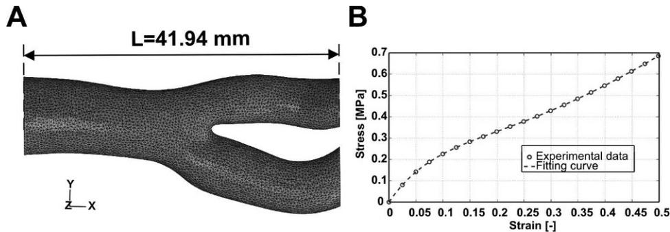
**Figure 2** ♦ (A) 3D reconstruction (triangulated surface) of the silicone artery pre-stenting. (B) Adopted stress-strain curve for silicone material and related data fitting curve.
