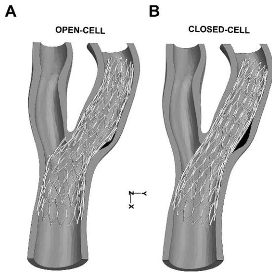
**Figure 7** ♦ Stent/vessel configurations obtained by FEA of CAS for the (A) open-cell and (B) closed-cell designs. The gap between the stent and the vessel wall is in black.
