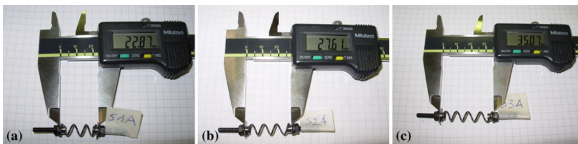
Fig. 3 Tested superelastic spring specimens. (a) S1A (b) S2A (c) S3A
