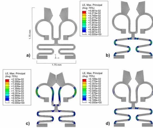
**Fig. 8:** Finite element analysis of micro-gripper: a) starting configuration; b) memorization step of linear actuator; c) heating of linear actuator and consequent actuation of the gauge; d) heating of gauge actuator with consequent re-opening. Contour plot of maximum principal logarithmic strain is reported.
