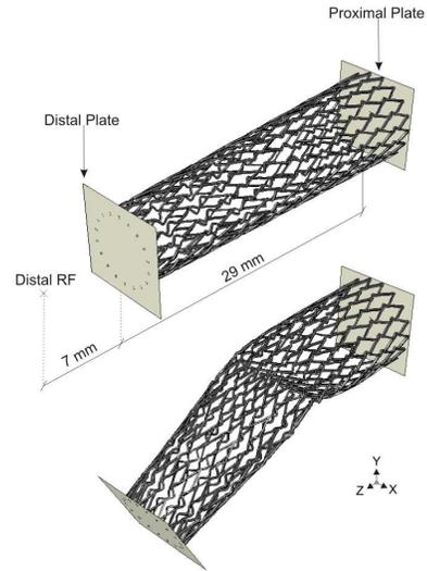
**Fig. 10:** Flexibility test of Nitinol stent; initial configuration (top); final bent configuration (bottom).
