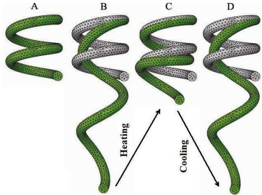
**Fig. 5:** Spring actuator: A) initial geometry; B) deformed shape due to the weight application at  $T = -25$  °C; C) spring shape recovery and weight lifting due to heating to  $T = 100$  °C; D) spring stretching due to cooling to  $T = -25$  °C.
