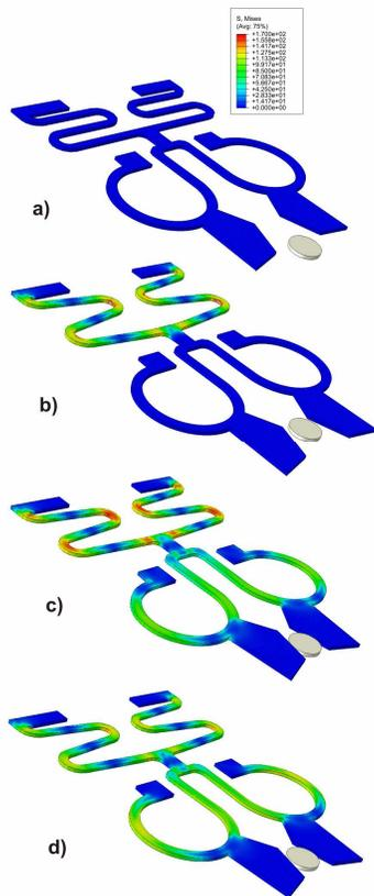
**Fig. 9:** Simulation of micro-gripper with a sample: a) starting configuration; b) memorization step; c) heating of linear actuator and sample gripping; d) heating of rotary actuator with consequent re-opening. von Mises stress [MPa] distribution in the micro-gripper are depicted in the contour plot.
