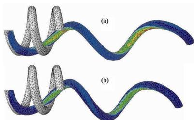
**Fig. 3:** Shape memory effect: deformed shape a) under maximum load b) after unloading.
