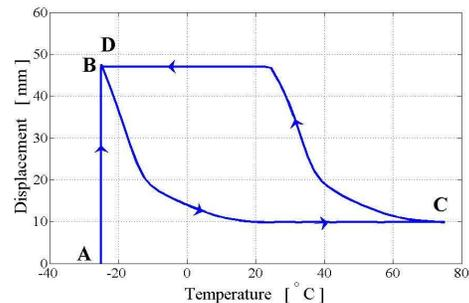
**Fig. 7:** Vertical displacement of the lower loaded end of spring versus temperature variation.
