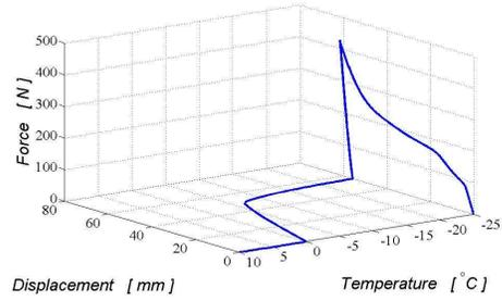
**Fig. 4:** Force-displacement diagram for the SMA spring: shape memory effect.
