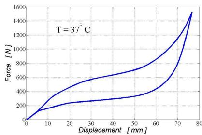
**Fig. 2:** Force-displacement diagram for the SMA spring: pseudo-elasticity
