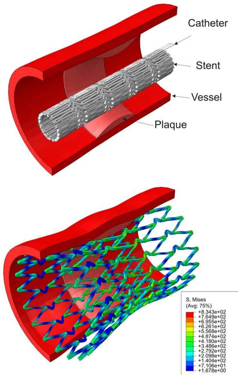
**Fig. 11:** Simulation of stent implant in a narrowed vessel; stent crimped in the catheter (top); stent delivered in the vessel. Von Mises stress [MPa] distribution in stent after the deployment are depicted in the contour plot (bottom).
