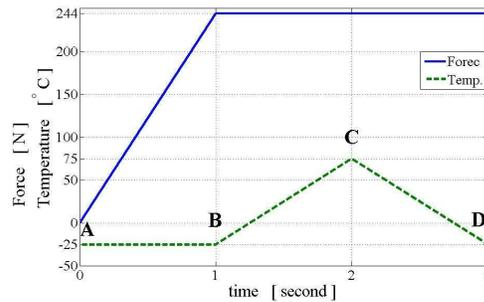
**Fig. 6:** Loading history during simulation.
