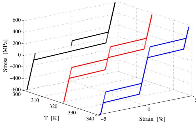
Fig. 1. Model response for tension-compression uniaxial loading at constant temperature.
