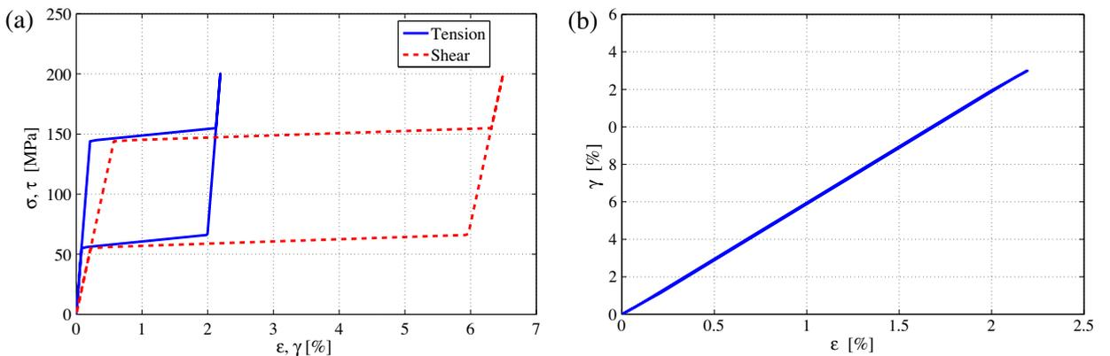
Fig. 5. Model prediction for proportional path 2: (a) stress–strain curves, (b) axial–shear strain response.
