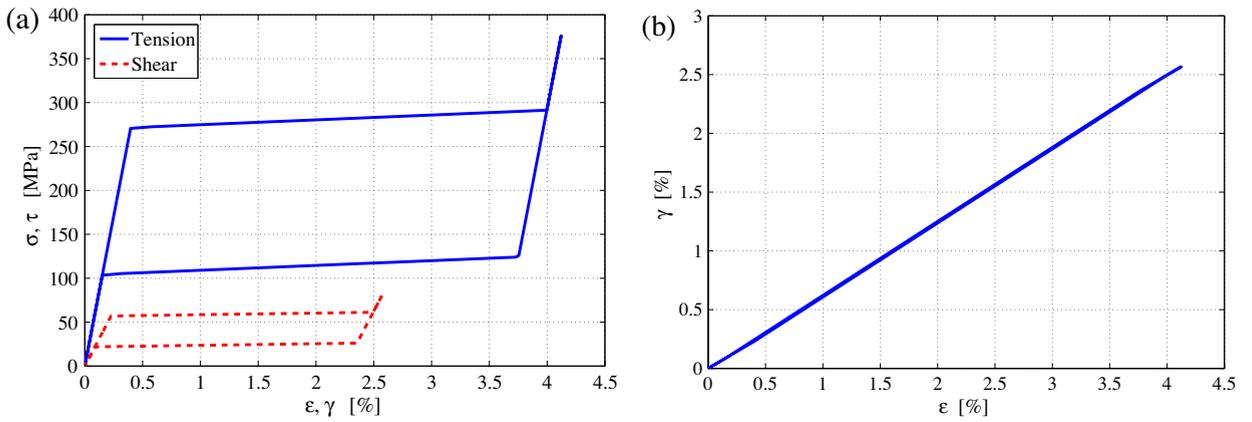
Fig. 4. Model prediction for proportional path 1: (a) stress–strain curves, (b) axial–shear strain response.
