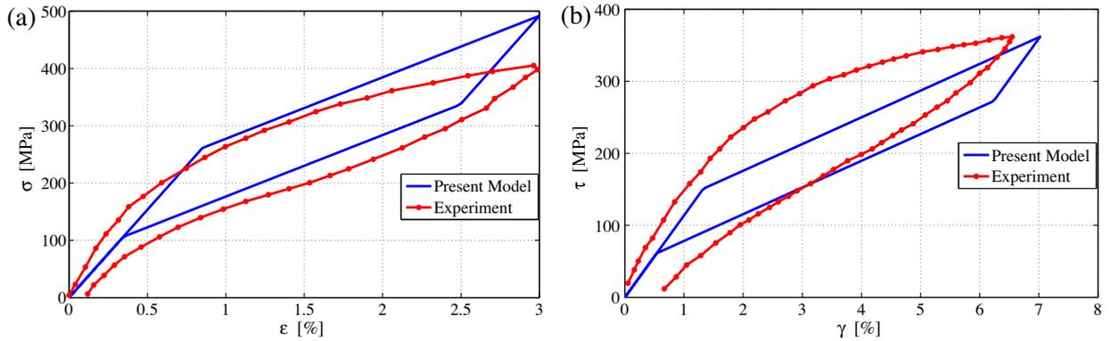
Fig. 7. Model prediction compared to the experimental data by Sittner et al. (1995): (a) uniaxial tension, (b) torsion.
