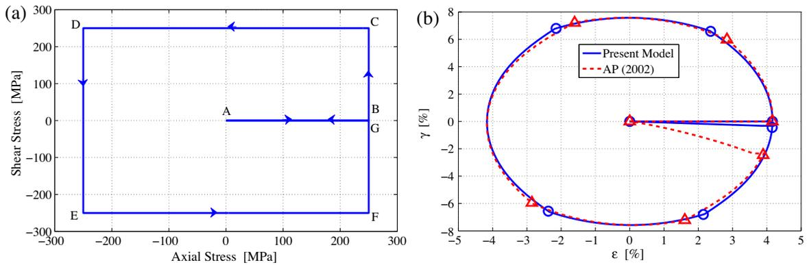
Fig. 6. Biaxial non-proportional loading: (a) axial-shear stress path, (b) comparison of model predictions for axial-shear strain response.
