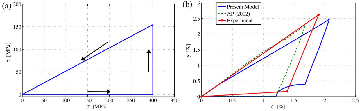
Fig. 9. Proposed model prediction and comparison with AP (2002) and experimental results (Sittner et al., 1995): (a) axial-shear triangle-shaped stress path, (b) axial-shear strain response.
