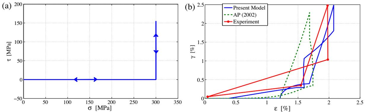
Fig. 10. Proposed model prediction and comparison with AP (2002) and experimental results (Sittner et al., 1995): (a) axial-shear L-shaped stress path, (b) axial-shear strain response.
