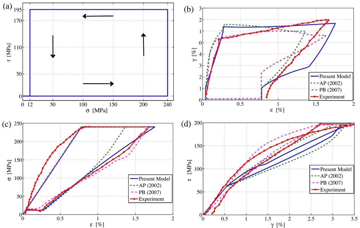
Fig. 8. Comparison between model predictions and experimental data (Sittner et al., 1995): (a) non-proportional biaxial tension-shear path, (b) axial-shear strain response, (c) axial stress-axial strain response, (d) shear stress-shear strain response.
