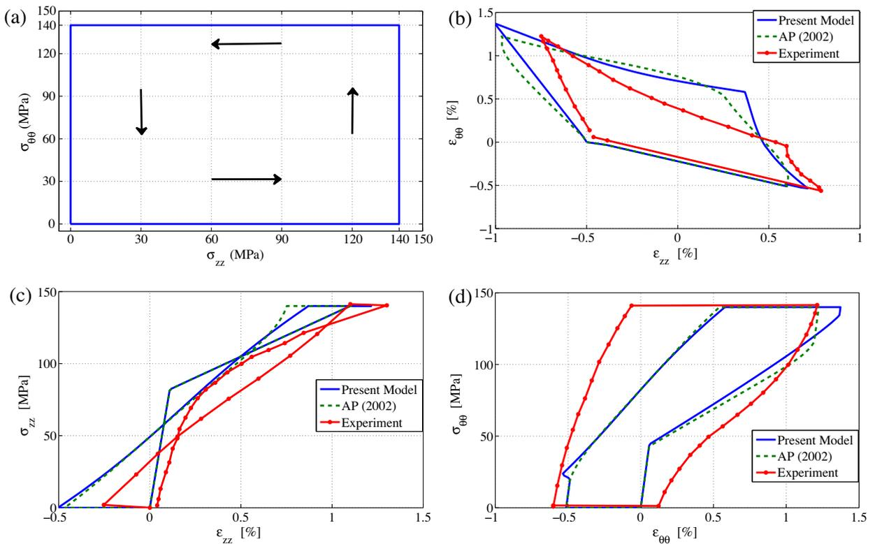
Fig. 12. Comparison between simulation and experimental results (Bouvet et al., 2002): (a) non-proportional biaxial loading path, (b) corresponding strain path, (c) axial stress–strain curve, (d) hoop stress–strain curve.
