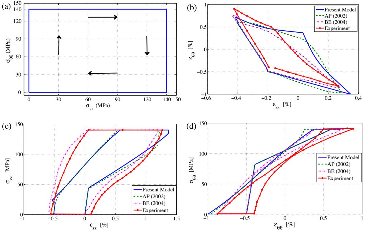
**Fig. 13.** Comparison between simulation and experimental results (Bouvet et al., 2004): (a) non-proportional biaxial loading path, (b) corresponding strain path, (c) axial stress–strain curve, (d) hoop stress–strain curve.
