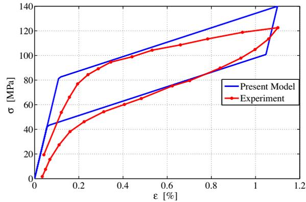
Fig. 11. Uniaxial tension behavior predicted by the model and comparison with experimental results from Bouvet et al. (2004).
