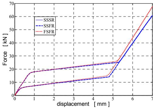
Figure 2. force-displacement diagram and comparison of different formulations under tension test.
