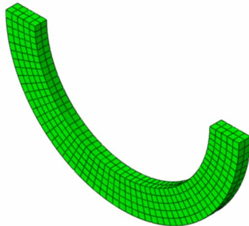
Figure 5. geometry and mesh description in the arc-shaped beam example under an out of plane force.
