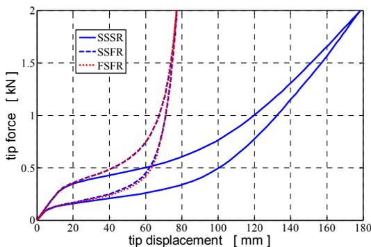
Figure 4. force-tip displacement diagram for the cantilever beam and different formulations comparison.
