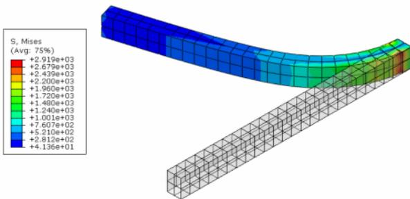
Figure 3. the cantilever beam under tip force, deformed shape when FSFR formulation is used.
