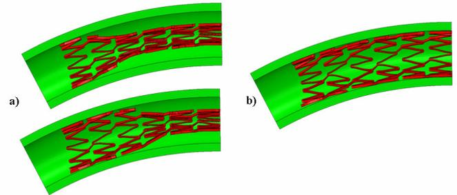
**Figure 4. Stent expansion in a curved vessel: a) partially deployed stent; b) fully deployed stent.**
