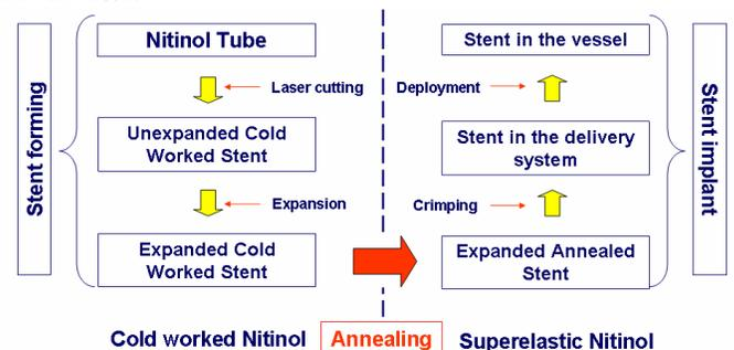
**Figure 1. Workflow of stent design forming and implant**
