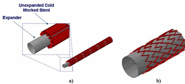
**Figure 2. Laser-cut stent and expander: a) closed configuration; b) open configuration.**
