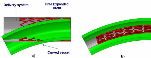
**Figure 3. Stent and delivery system: a) undeformed configuration; b) crimped/bent configuration.**
