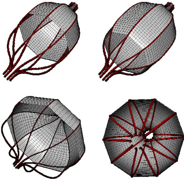
**Figure 2. Design variants of the Angioguard model: original 4 mm device with 50% membrane coverage (top left), 80% membrane covered 4 mm filter (top right), 8 mm device with 50% membrane coverage (bottom left) and 10 strut variant (bottom right).**
