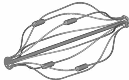
**Figure 1. 3D reconstruction of microCT scan of a 4 mm Angioguard filter (membrane not visible)**
