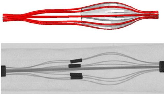
**Figure 3. Finite Element simulation (top panel) and microCT image (bottom panel) of partially inserted/released filter into/from the delivery sheath**
