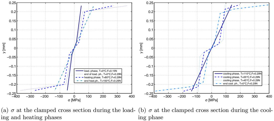
Figure 3: Stress responses along the clamped end cross section.
