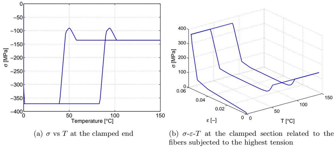
Figure 2:  $\sigma$  and  $\sigma$ - $\epsilon$  at the clamped section as function of temperature
