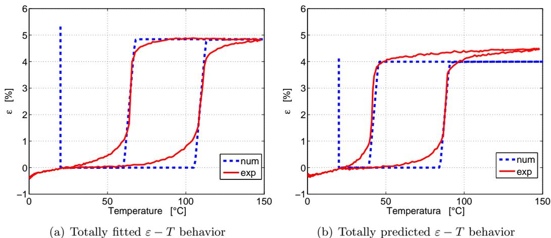
Figure 1: Numerical and experimental tests for two different uniaxial tensile loads
