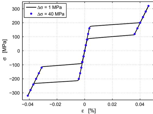
Fig. 4. Stress-driven test at  $T = 293$  K.
