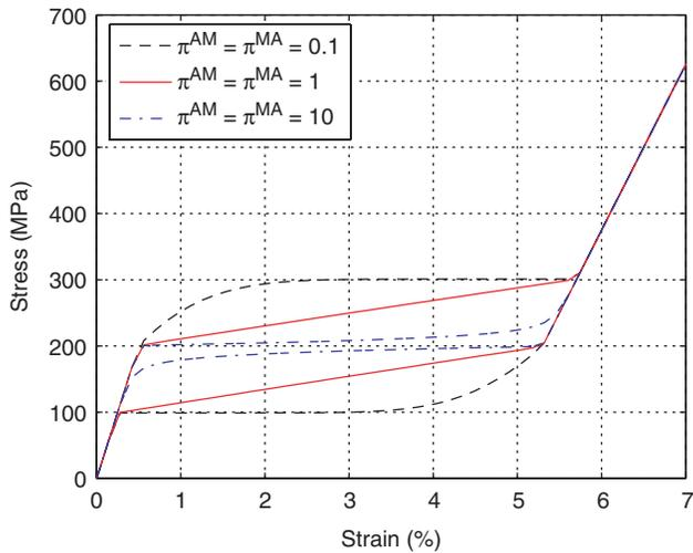
**Figure 2.** Power rules: stress-strain relationship for quasi-static loading-unloading conditions. Setting speed parameters  $\pi^{AM}$  and  $\pi^{MA}$  equal to 1 leads to linear rules.
