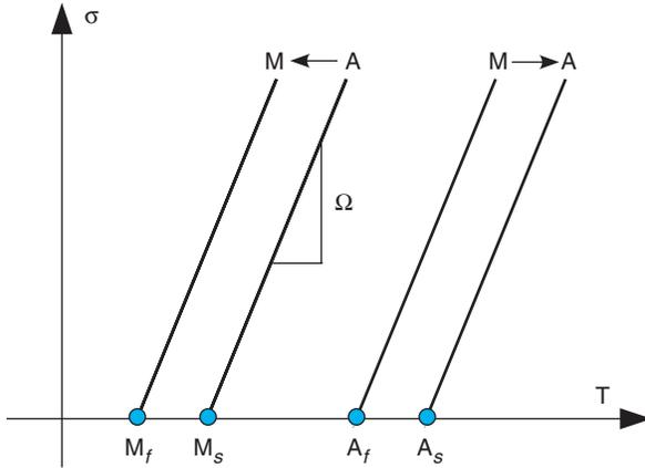
**Figure 1.** Phase transformation zones ( $A$  = austenite,  $M$  = martensite,  $\Omega$  = slope).  $A_s$ ,  $A_f$ ,  $M_s$ , and  $M_f$  are the temperature levels at which the forward ( $A \rightarrow M$ ) and reverse ( $M \rightarrow A$ ) phase transformation starts and finishes, respectively.
