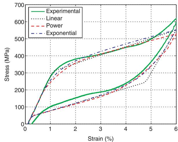
**Figure 9. Dynamic loading conditions: experimental data (set 1) vs numerical results.**
