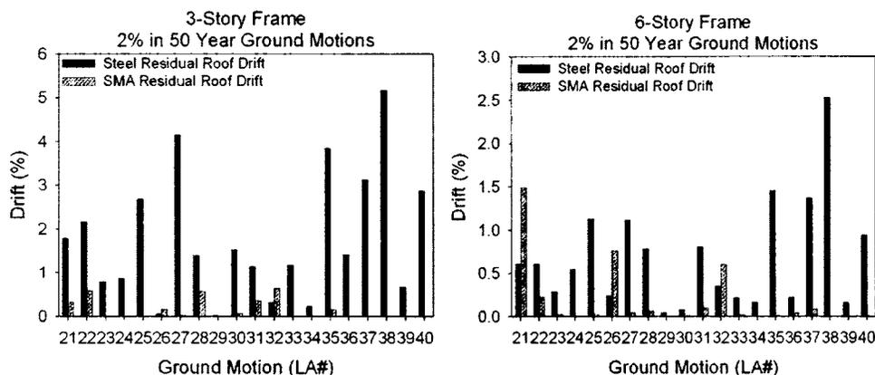
Fig. 10. Residual roof drift of the three- and six-story frames for the 2% probability of exceedence in 50 years ground motions
