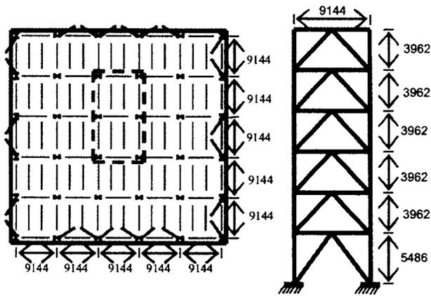
**Fig. 3.** Plan and elevated view of the six-story frame (mm) with the penthouse indicated with a dashed line
