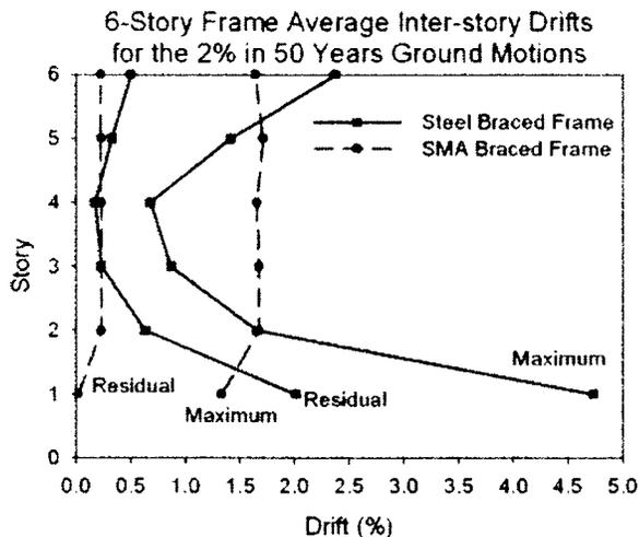
**Fig. 11.** Maximum and residual interstory drifts with respect to each floor level for the six-story frame undergoing the 2% probability of exceedence ground motions
