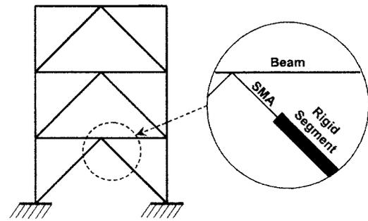
**Fig. 4.** Detail of the SMA brace installed in the three-story frame
