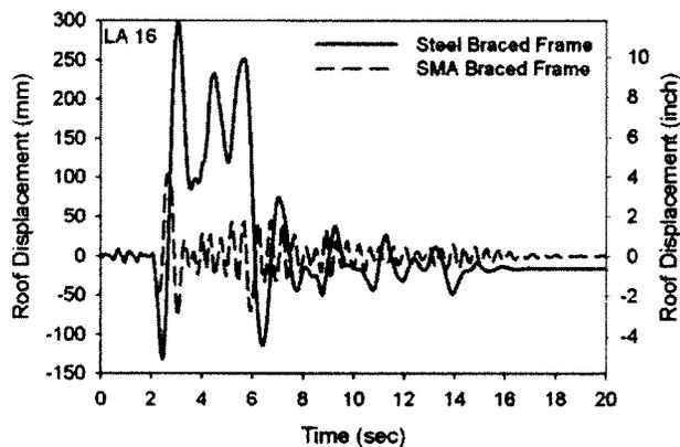
**Fig. 7.** Displacement time histories of the top floor when the three-story building undergoes the LA16 earthquake
