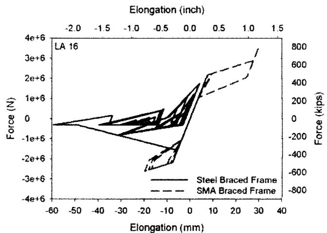
**Fig. 8.** Force-displacement relationship exhibited by the left brace of the first floor when the three-story building is hit by the LA16 earthquake
