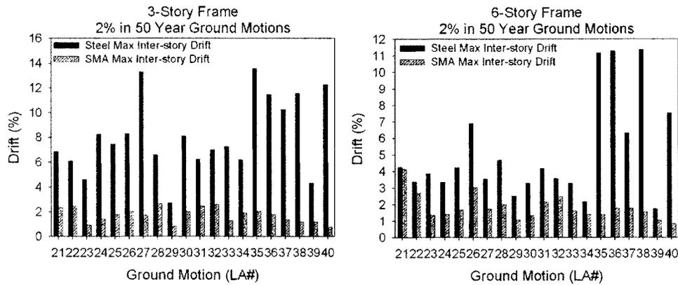
Fig. 9. Maximum interstory drift of the three- and six-story frames for the 2% probability of exceedence in 50 years ground motions
