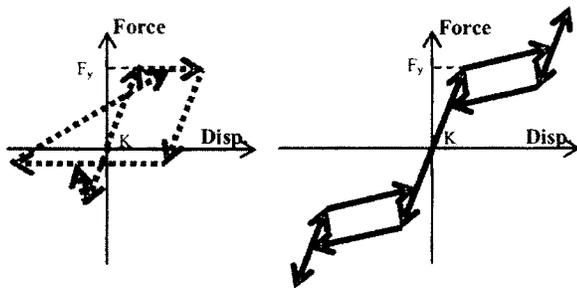
Fig. 5. Force–displacement relationship of: (a) buckling-allowed steel elements; (b) SMA members
