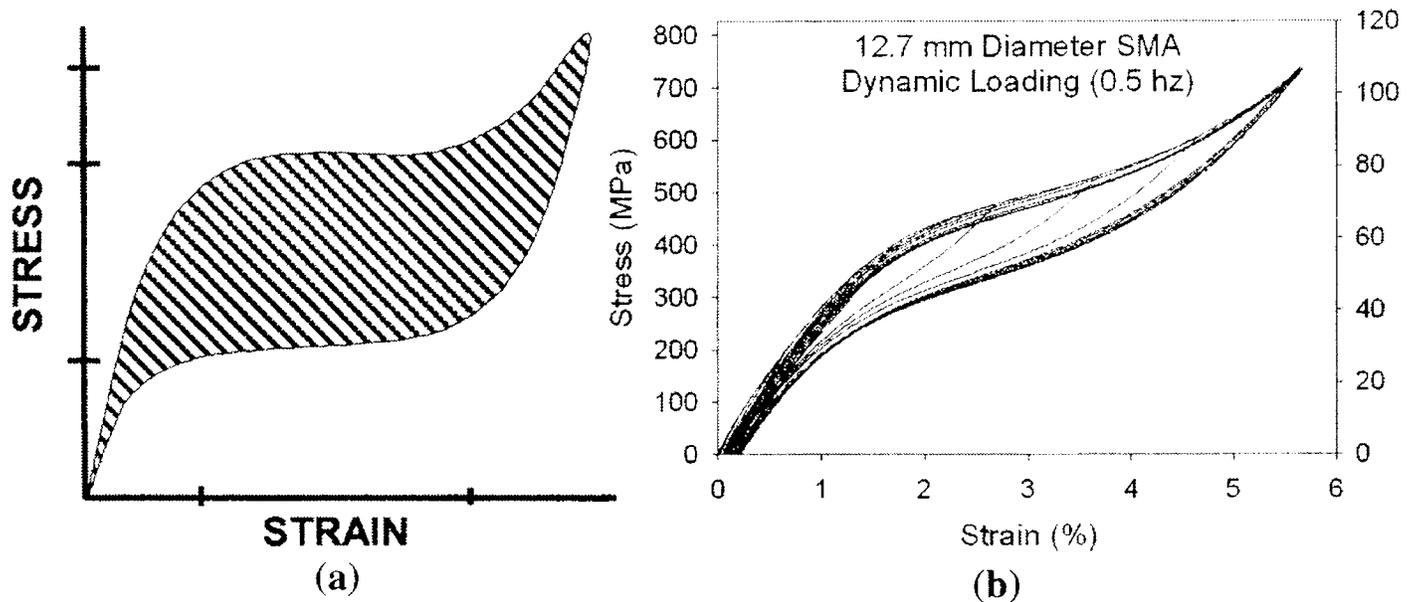
**Fig. 1.** (a) Idealized superelastic SMA behavior; (b) experimental results from cyclic tensile tests on a 12.7 mm diameter SMA bar (DesRoches et al. 2004)
