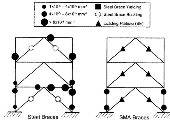
Fig. 6. Member yielding during the LA16 ground motion for the steel and SMA braced frames
