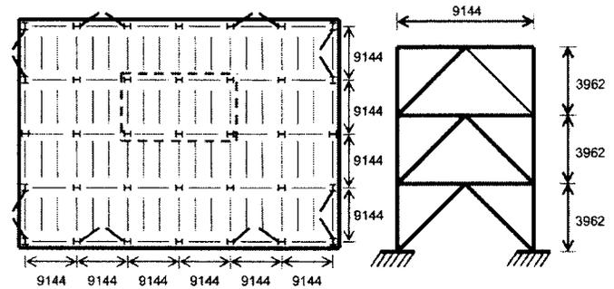
Fig. 2. Plan and elevated view of the three-story frames (mm) with the penthouse indicated with a dashed line
