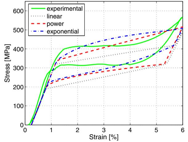
**Figure 15.** Dynamic loading conditions: experimental data (set 3) versus numerical results.
