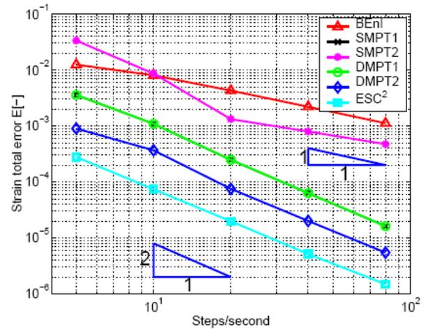
Fig. 2 Pointwise stress-strain test. Stress and strain total error versus number of steps per second.
