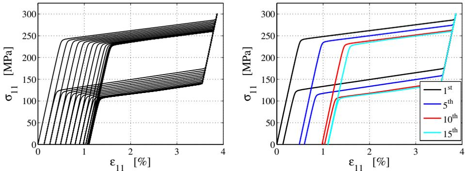
Fig. 8. Uniaxial tests: 15 tension cycles with saturating permanent inelasticity, including degradation effect ( $H = 1.5 \times 10^4$  MPa,  $A = 2 \times 10^3$  MPa,  $\kappa = 2\%$ ,  $T = 298$  K). Axial stress–axial strain output.
