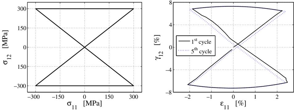
Fig. 10. Biaxial tests: non-proportional hourglass-shaped test ( $H = 1.5 \times 10^4$  MPa,  $A = 4 \times 10^3$  MPa,  $\kappa = 10\%$ ,  $T = 298$  K).  $\sigma_{11} - \sigma_{12}$  input (left) and 1st and 5th cycle  $\epsilon_{11} - \gamma_{12}$  output (right).
