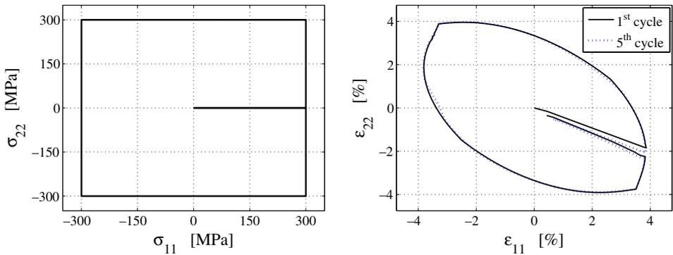
Fig. 11. Biaxial tests: non-proportional square-shaped test ( $H = 1.5 \times 10^4$  MPa,  $A = 4 \times 10^3$  MPa,  $\kappa = 10\%$ ,  $T = 298$  K).  $\sigma_{11} - \sigma_{22}$  input (left) and 1st and 5th cycle  $\epsilon_{11} - \epsilon_{22}$  output (right).
