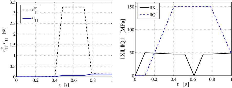
Fig. 5. Uniaxial tests: single tension cycle with permanent inelasticity ( $H = 0$  MPa,  $A = 0$  MPa,  $\kappa = 2\%$ ,  $T = 298$  K). Output histories for  $e_{11}^{tr}$  and  $q_{11}$  (left) and  $\|X\|$  and  $\|Q\|$  (right).
