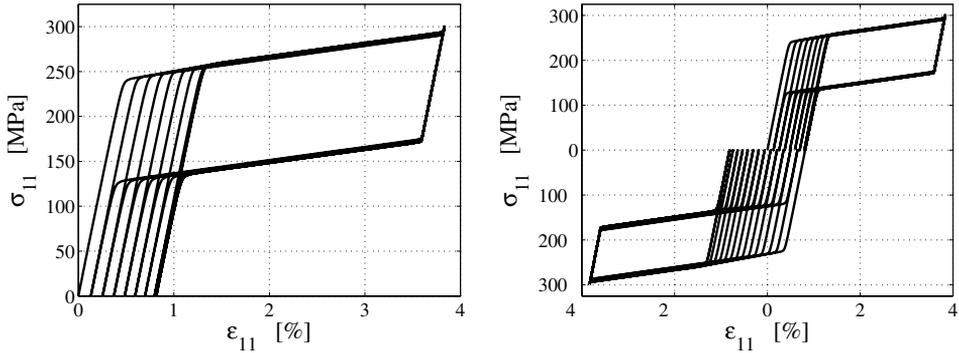
Fig. 7. Uniaxial tests: 10 tension cycles (left) and 10 tension followed by 15 compression cycles (right) with saturating permanent inelasticity ( $H = 1.5 \times 10^4$  MPa,  $A = 0$  MPa,  $\kappa = 2\%$ ,  $T = 298$  K). Axial stress–axial strain output.
