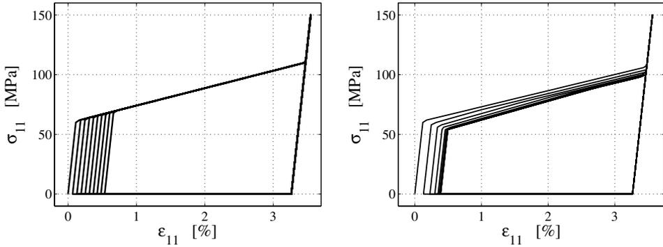
Fig. 9. Uniaxial tests: multiple (10) tension cycles at  $T = M_f$ , each one followed by heating strain recovery, with  $H = 0$  MPa,  $A = 0$  MPa (left) and  $H = 1.5 \times 10^4$  MPa,  $A = 2 \times 10^3$  MPa (right) and  $\kappa = 2\%$ . Axial stress–axial strain output.
