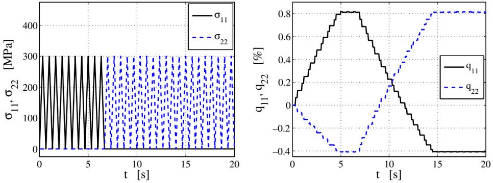
Fig. 12. Combined uniaxial tests: 10 tension cycles in direction 1 followed by 20 in direction 2 ( $H = 1.5 \times 10^4$  MPa,  $A = 0$  MPa,  $\kappa = 2\%$ ,  $T = 298$  K). Stress input histories (left) and  $q_{11}$  and  $q_{22}$  output histories (right).
