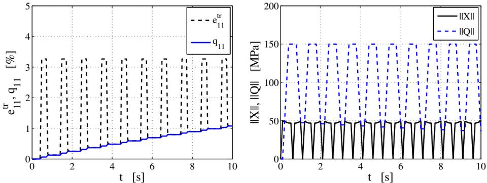
Fig. 6. Uniaxial tests: 10 tension cycles with permanent inelasticity ( $H = 0$  MPa,  $A = 0$  MPa,  $\kappa = 2\%$ ,  $T = 298$  K). Output histories for  $e_{11}^{tr}$  and  $q_{11}$  (left) and  $\|X\|$  and  $\|Q\|$  (right).
