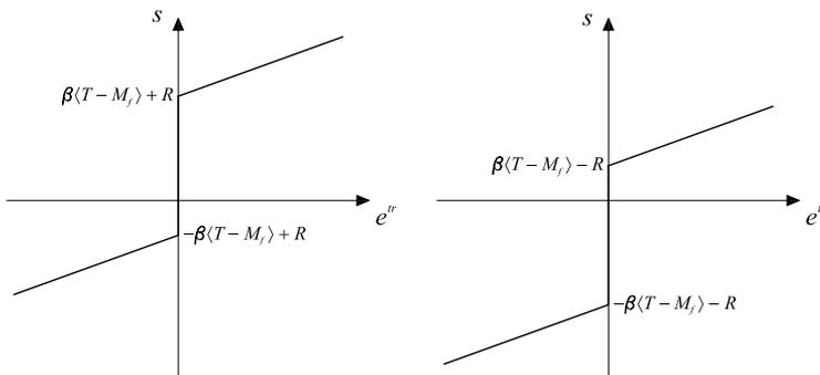
Fig. 2. Plots of  $s = s(e^{tr})$  in the cases of unloading from compression (left) and from tension (right).
