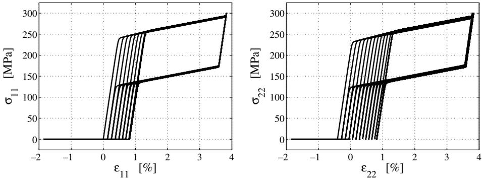
Fig. 13. Combined uniaxial tests: 10 tension cycles in direction 1 followed by 20 in direction 2 ( $H = 1.5 \times 10^4$  MPa,  $A = 0$  MPa,  $\kappa = 2\%$ ,  $T = 298$  K).  $\sigma_{11} - \epsilon_{11}$  output (left) and  $\sigma_{22} - \epsilon_{22}$  output (right).
