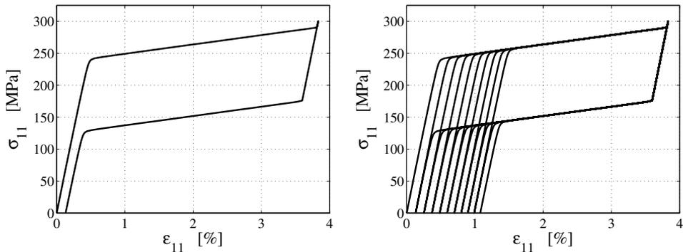
Fig. 4. Uniaxial tests: tension cycles with permanent inelasticity ( $H = 0$  MPa,  $A = 0$  MPa,  $\kappa = 2\%$ ,  $T = 298$  K). Axial stress–axial strain output for single (left) and multiple (right) tension loops.
