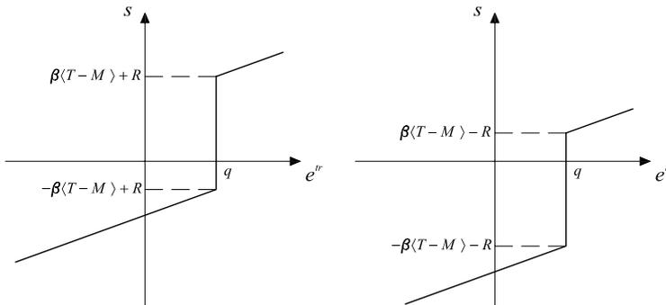
Fig. 3. Translated plots of  $s = s(e^{\text{tr}})$  in the cases of unloading from compression (left) and from tension (right).
