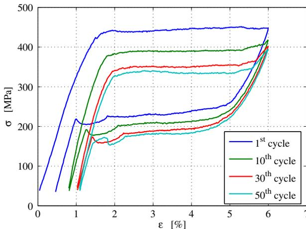
Fig. 1. Experimental results on a SMA Ni–Ti wire. Cyclic tension test: stress versus strain up to 6% strain.
