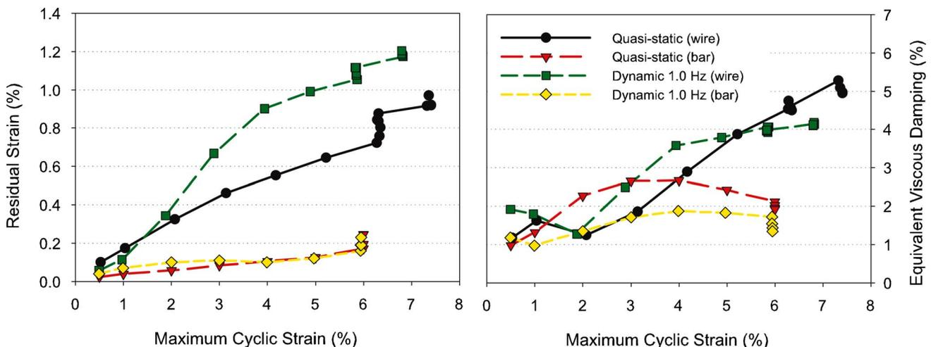
Fig. 3 Cyclic properties comparison of NiTi shape memory alloys: (a) residual strain and (b) equivalent viscous damping
