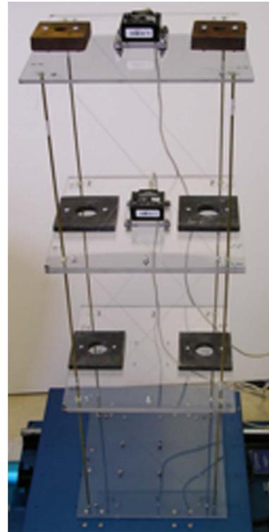
Fig. 4 Proof-of-concept shake table model with 0.254 mm (0.01 in.) diameter SMA braces
