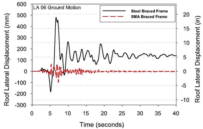
Fig. 9 Displacement time history of the roof experienced in the three-story frame excited by the LA06 record
