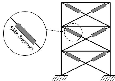
Fig. 7 Detail of the innovative SMA braces in the three-story frame
