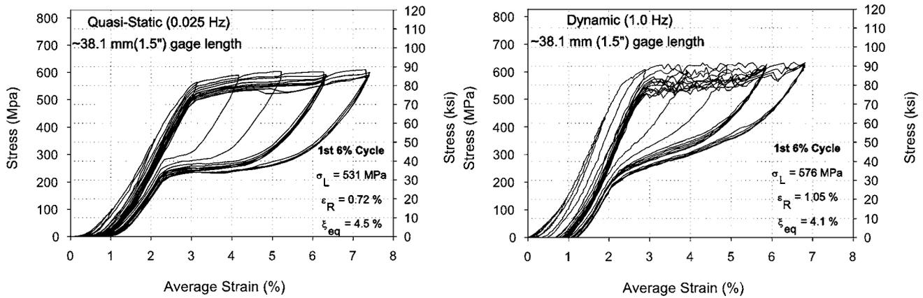
**Fig. 1** Stress-strain curves for 0.254 mm (0.01 in.) diameter NiTi shape memory alloys tested at (a) 0.025 Hz and (b) 1.0 Hz loading rates
