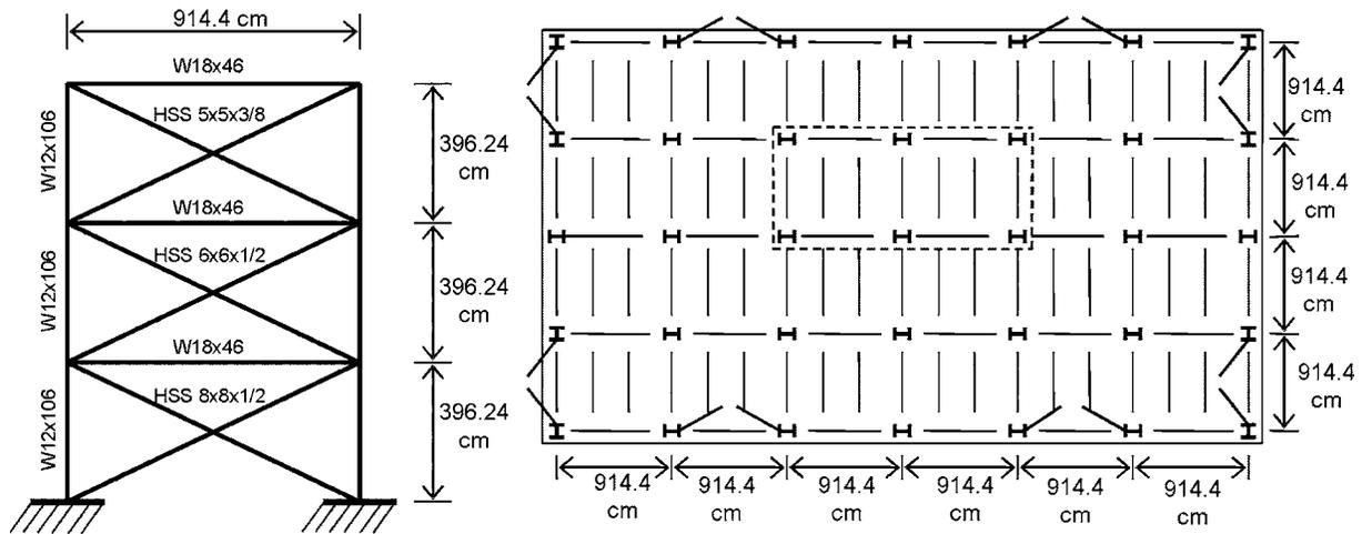
Fig. 6 Elevation and plan view of the three-story frame
