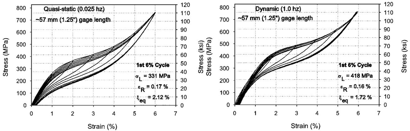
Fig. 2 Stress-strain curves for 12.7 mm (0.5 in.) diameter NiTi shape memory alloys tested at (a) 0.025 Hz and (b) 1.0 Hz loading rates [13]
