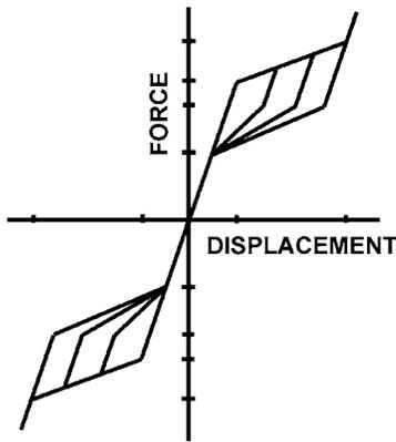
Fig. 8 Force-displacement relationship for the SMA braces
