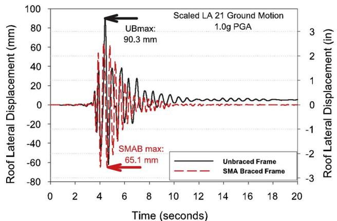
Fig. 5 Analytical displacement time history of the roof for the proof-of-concept model undergoing the LA21 ground motion scaled to 1.0 PGA
