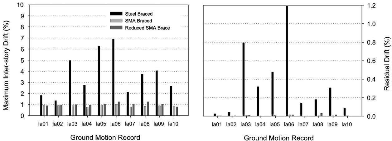
Fig. 11 (a) Maximum inter-story drift and (b) residual drift of the top floor exhibited by the three-story steel braced frame with either conventional steel braces, innovative SMA braces, or innovative SMA braces with a reduced cross-sectional area
