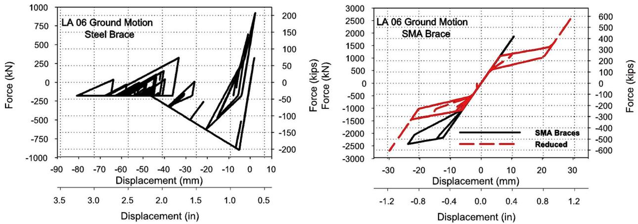
Fig. 10 Force-displacement relationship experienced by one of the bottom braces excited by the LA06 record: (a) steel brace and (b) SMA brace
