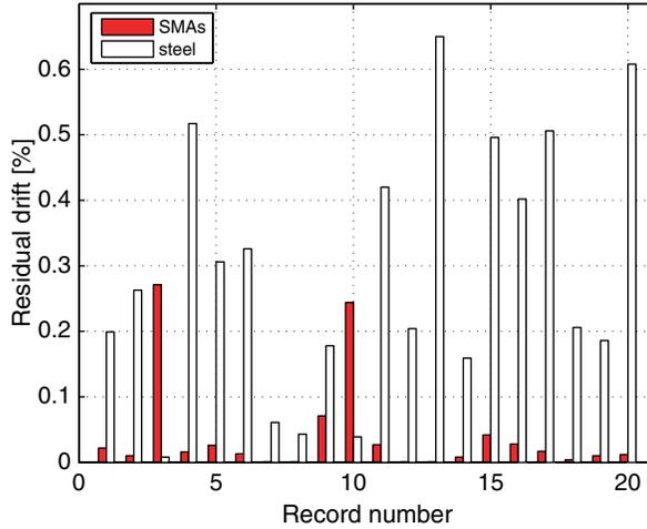
Fig. 12. Residual drift of the top floor exhibited by the six-storey frame equipped with either buckling-restrained steel braces or superelastic SMA braces.
