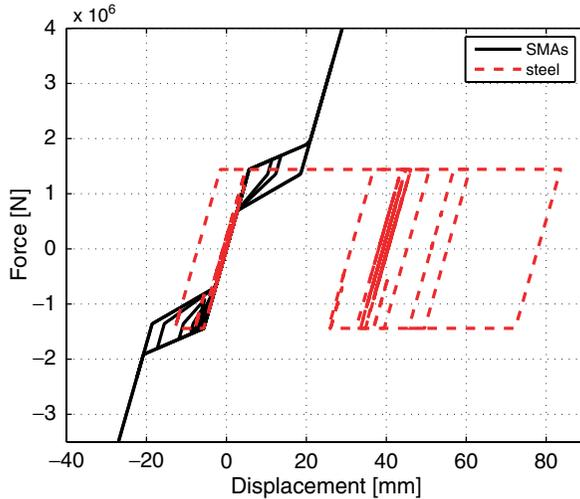
Fig. 8. Force-displacement relationship exhibited by the lower left brace installed in the three-storey frame undergoing ground motion LA6 scaled to a value of PGA of 0.67  $g$ . Note the different hysteresis loops between structural steel and superelastic SMAs.
