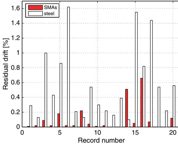
Fig. 10. Residual drift of the top floor exhibited by the three-storey frame equipped with either buckling-restrained steel braces or superelastic SMA braces.
