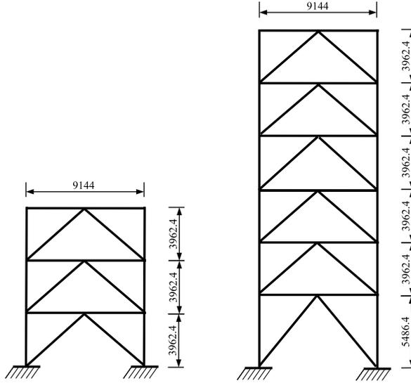
Fig. 3. Elevation view of the three- and six-storey frame. Dimensions are expressed in mm.
