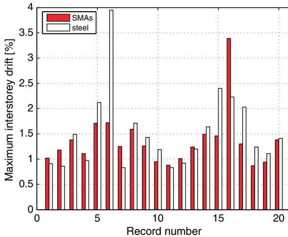
Fig. 9. Maximum interstorey drift exhibited by the three-storey frame equipped with either buckling-restrained steel braces or superelastic SMA braces.
