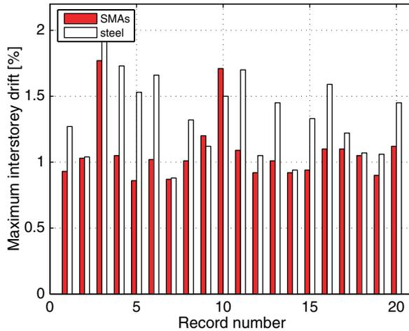
Fig. 11. Maximum interstorey drift exhibited by the six-storey frame equipped with either buckling-restrained steel braces or superelastic SMA braces.
