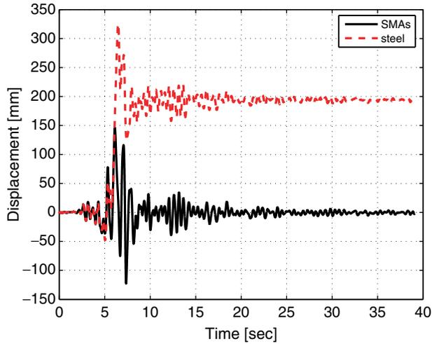
Fig. 7. Displacement time-history exhibited by the top floor of the three-storey frame equipped with either buckling-restrained steel braces or superelastic SMA braces undergoing ground motion LA6 scaled to a value of PGA of  $0.67g$ .
