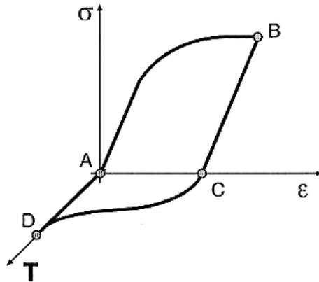
Fig. 2. Shape-memory effect. At the end of a loading-unloading path ( $ABC$ ) performed at a constant low temperature, the material presents residual deformations ( $AC$ ) which can be recovered through a thermal cycle ( $CDA$ ).
