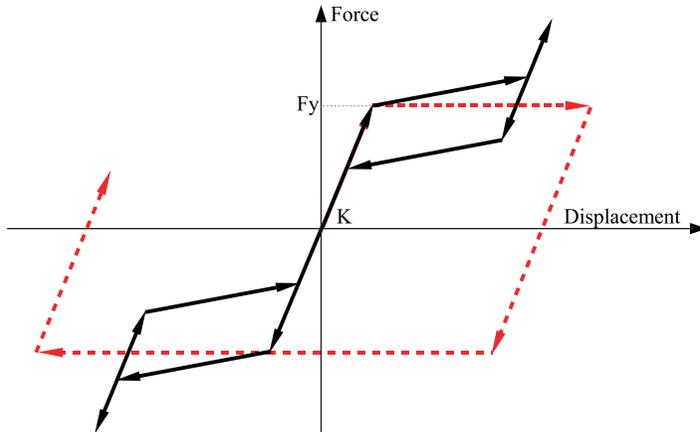
Fig. 4. Material models: buckling-restrained steel (dashed line) and superelastic SMAs (continuous line).
