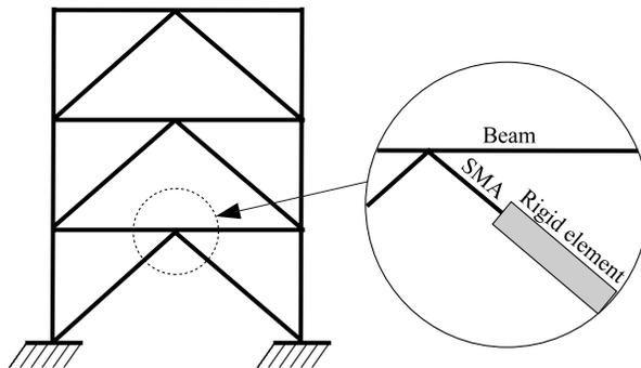
Fig. 5. Particular of the superelastic SMA brace installed in the three-storey frame.
