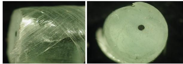
**Figure 1.** A CF-GFRP rod made of an internal unidirectional carbon fibre rod inserted in a glass fibre bundle: (a) transverse sight, (b) section.
