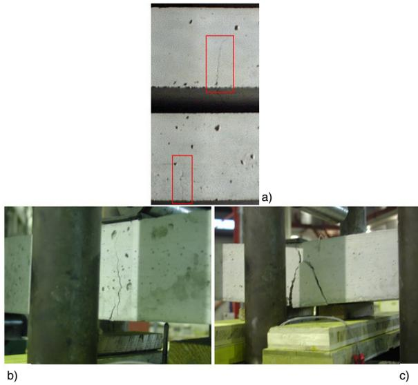
**Figure 5.** (a) Some cracks appearing on beam 1 immediately after load application; (b) beam 1 after rod 2 failure and (c) beam 1 at failure.
