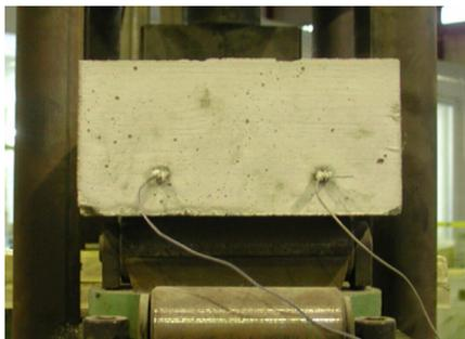
**Figure 3.** A picture of the section of a self-sensing CF-GFRP rods reinforced beam.
