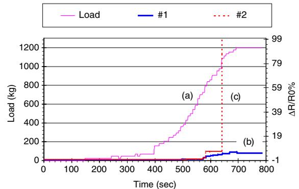
**Figure 4.** Mechanical and electrical results on beam 1: (a) load/ time curve; (b)  $\Delta R/R_0\%$ / time curve of self-sensing rod 1 and (c)  $\Delta R/R_0\%$ / time curve of self-sensing composite rod 2.
