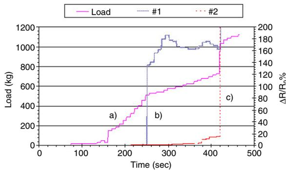
**Figure 6.** Mechanical and electrical results on beam 2: (a) load/time curve; (b)  $\Delta R/R_0\%$  time curve of self-sensing rod 1 and (c)  $\Delta R/R_0\%$  time curve of self-sensing rod 2.
