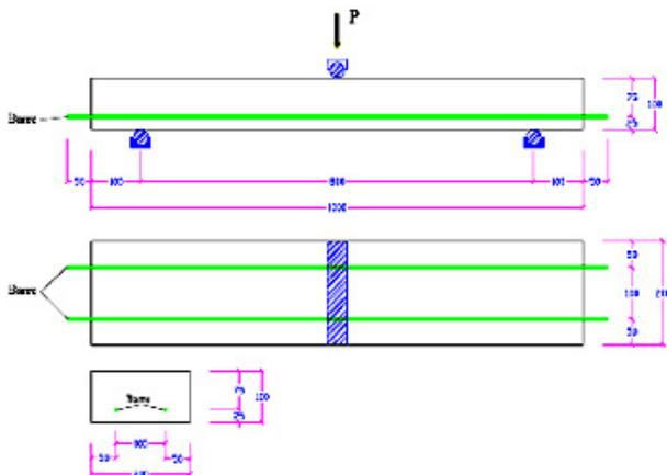
**Figure 2.** Beam design containing two reinforcing rods.
