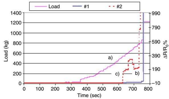
**Figure 7.** Mechanical and electrical results on beam 3: (a) load/time curve; (b)  $\Delta R/R_0\%$  time curve of self-sensing rod 1 and (c)  $\Delta R/R_0\%$  time curve of self-sensing rod 2.
