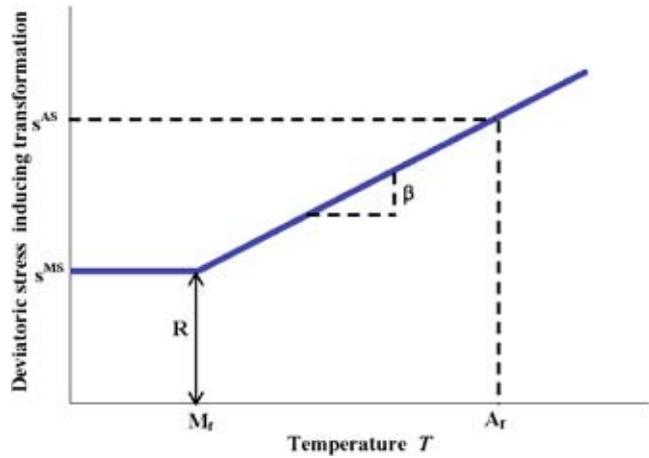
**Fig. 3 Stress deviatoric component inducing transformation-temperature relation.**  $s^{MS}$ =value of the stress deviatoric component inducing  $M \rightarrow S$  transformation at temperature  $T \leq M_f$ ;  $s^{AS}$ =value of the stress deviatoric component inducing  $A \rightarrow S$  transformation at temperature  $T = A_f$ .
