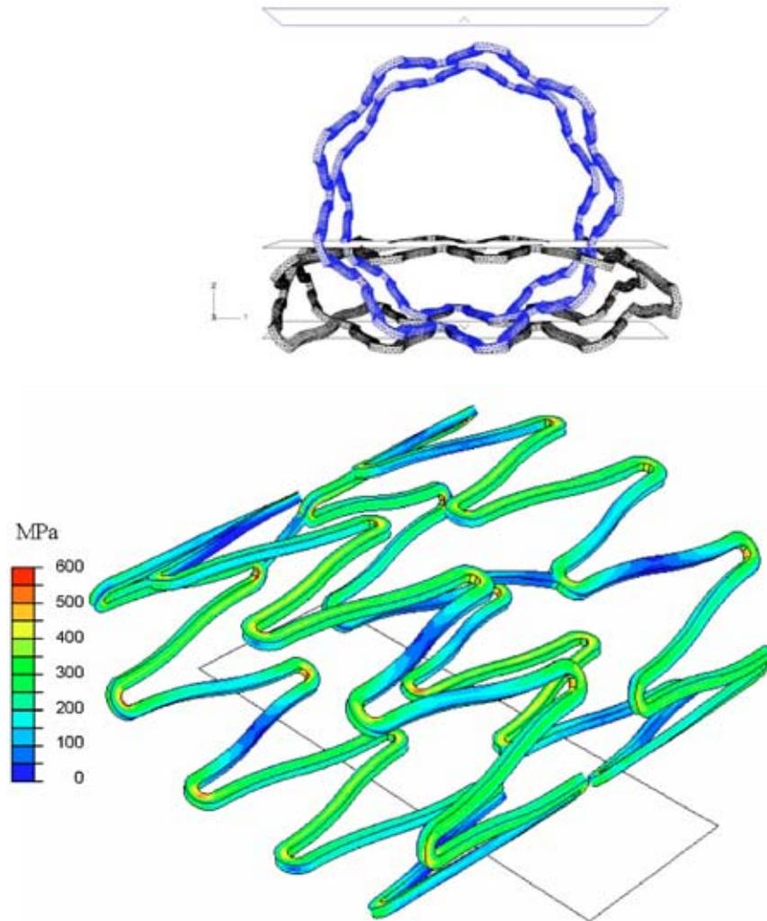
**Fig. 10 Numerical simulation: deformed (black) and undeformed (blue) configuration in a prospective view at the end of the loading step. In the lower panel the Von Mises stresses are depicted at the end of the loading step.**
