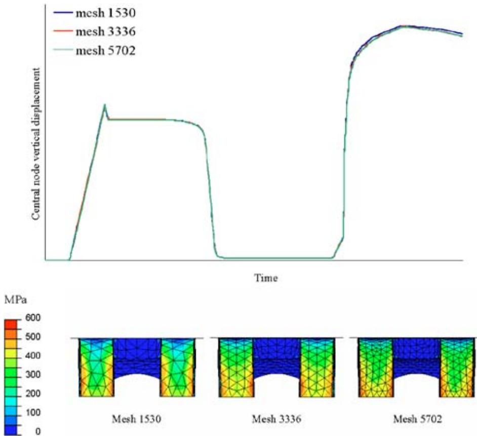
**Fig. 8 Results from the sensitivity analysis of the spacer model A: comparison between the displacement histories of a central node (upper panel) and the Von Mises stresses at the end of the loading path (lower panel) of three different meshes with 1530, 3336, and 5702 elements, respectively**
