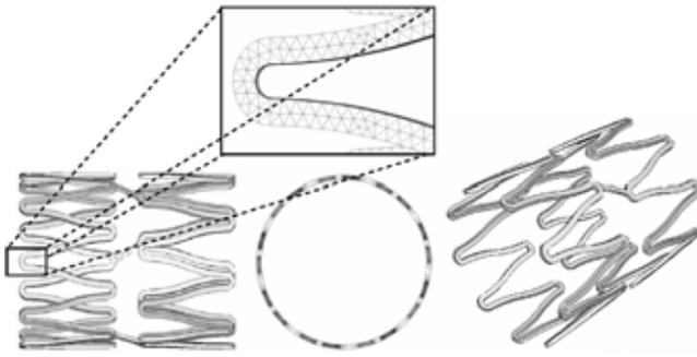
Fig. 5 CAD model of the Ni-Ti stent simulated
