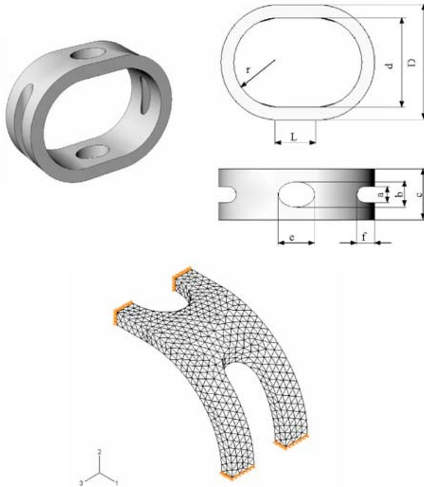
**Fig. 7 Three-dimensional CAD model of the spinal vertebrae spacer. Due to the symmetry only one fourth of the device is simulated. The mesh of the spacer and the boundary conditions are reported in the lower panel.**
