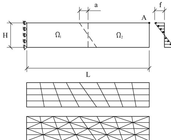
Fig. 8. Bending test. Problem geometry, boundary and loading conditions. Distorted  $4 \times 4$  meshes.
