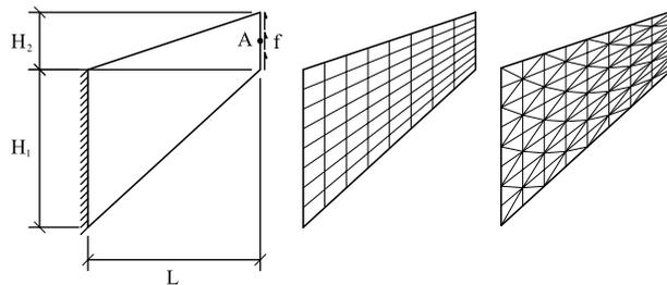
Fig. 9. Cook's membrane. Problem geometry, boundary and loading conditions.  $8 \times 8$  meshes.
