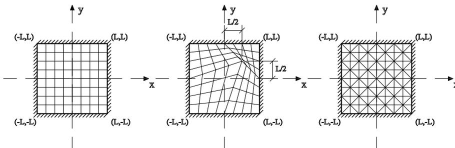
Fig. 1. Fully constrained block. Problem geometry and boundary conditions. Undistorted quadrilateral, distorted quadrilateral and triangular meshes.
