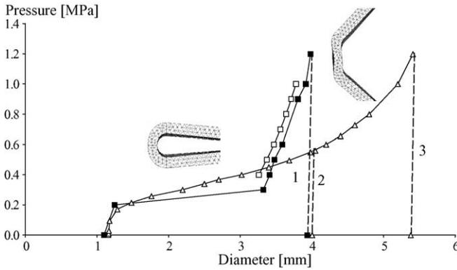
Fig. 4. Results from the FEM analysis (empty triangle), from the experimental test (solid squares) and data provided by the company (empty squares). The dotted lines represent the unload history at different values of inflating pressures both for the FEM and the experimental analyses. It should be noted that at 0.5 MPa the diameter reached by the stent is similar in the FEM simulation and the experimental test.
