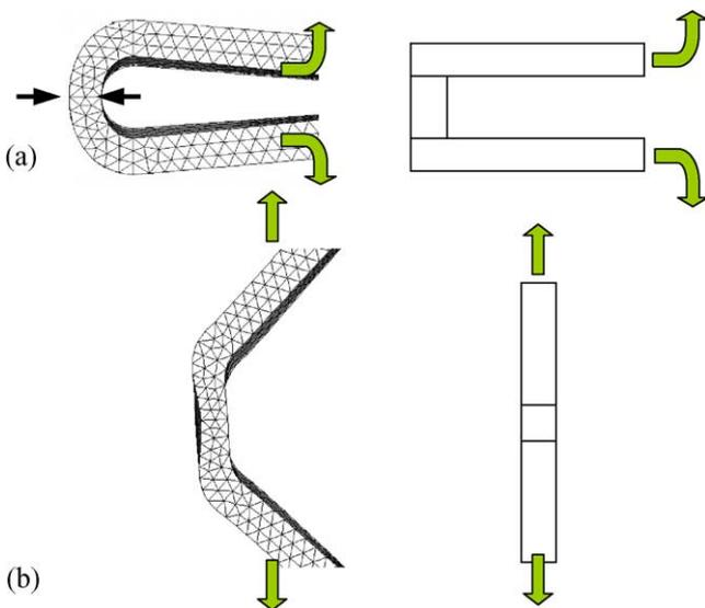
Fig. 5. Sketch of the ring stent like a cantilever under flexion before the expansion (a) and like beam subjected to tensile load after the expansion (b).
