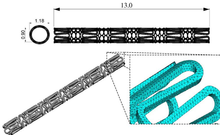
Fig. 1. 3D CAD model of the ‘Cordis BX Velocity’ stent. In the inset is depicted a particular of the mesh.
