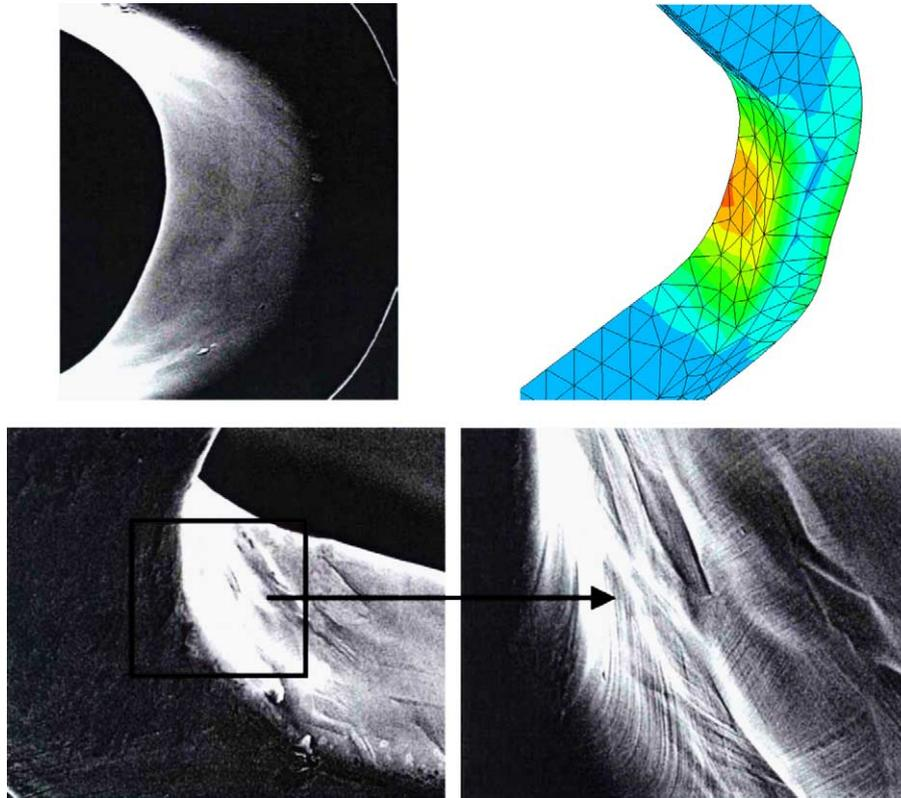
Fig. 6. Scanning electron microscopy (SEM) images and equivalent plastic deformation in the corresponding area of the FEM model. The enlargement in the area of the link shows clearly the areas of plastic deformation (Luders lines).
