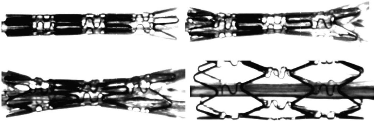
Fig. 2. Stent expansion as acquired by the optic estensometer at four different inflating pressures. It is possible to observe the expansion of the balloon in the distal zones of the stent before a uniform shape is reached.
