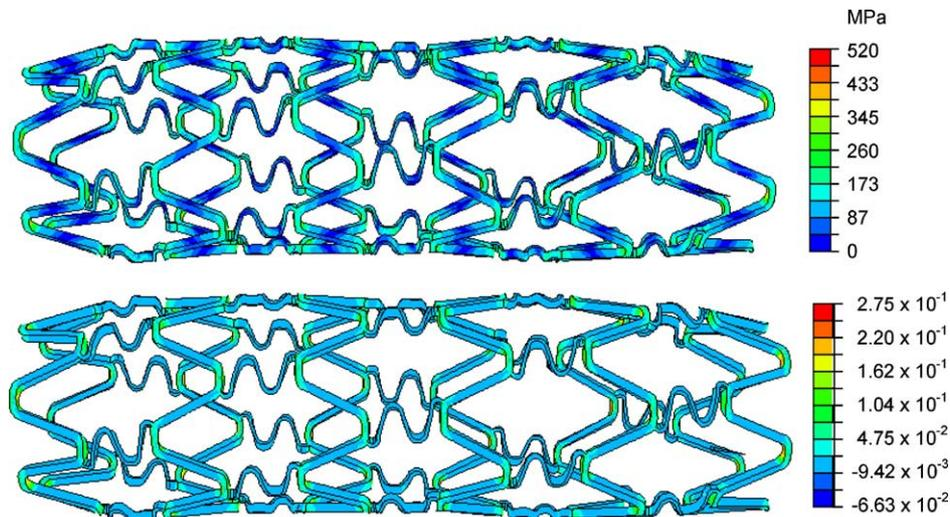
Fig. 3. von Mises stresses at the inflating pressure of 0.5 MPa (top) and equivalent plastic deformation after the load removal (bottom).
