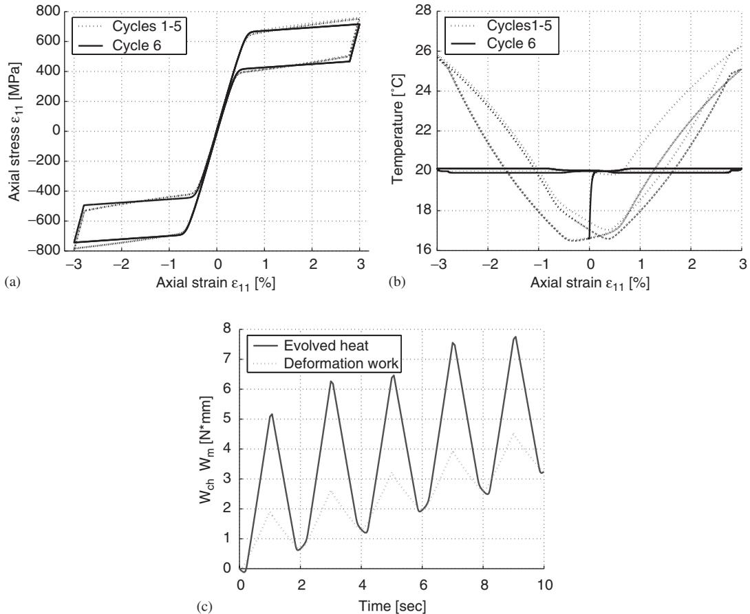
Figure 1. SMA specimen response under cyclic tension–compression test at different strain rates:  $5 \times 10^{-4} \text{ s}^{-1}$  in the first 5 cycles,  $5 \times 10^{-6} \text{ s}^{-1}$  in the last cycle. Comparison between the stress–strain curves (a) and the temperature–strain curves (b) of the 6 cycles. Comparison between the evolved heat and the deformation work during the first 2 cycles and half (c).
