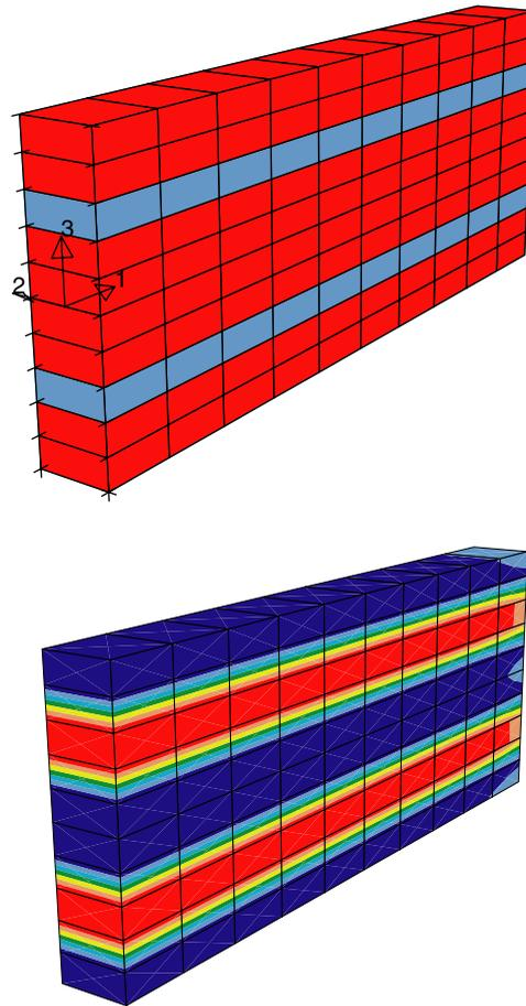
Figure 6. Model of hybrid composite with prestrained martensitic SMA wires (volume fraction  $v_w = 0.2$ ) embedded in a stiff polymeric matrix (Problem C) (upper part). Prestress induced in the cantilever by SMA constrained strain recovery (lower part).
