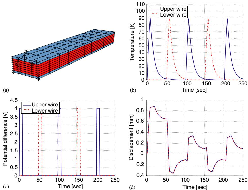
Figure 4. Model of hybrid composite with prestrained martensitic SMA wires (volume fraction  $v_w = 0.125$ ) surface mounted on soft polymeric matrix (Problem B) (a). Active shape control by SMA wire actuated through Joule effect: temperature time history (b); potential difference time history (c); free edge displacement time history (d).
