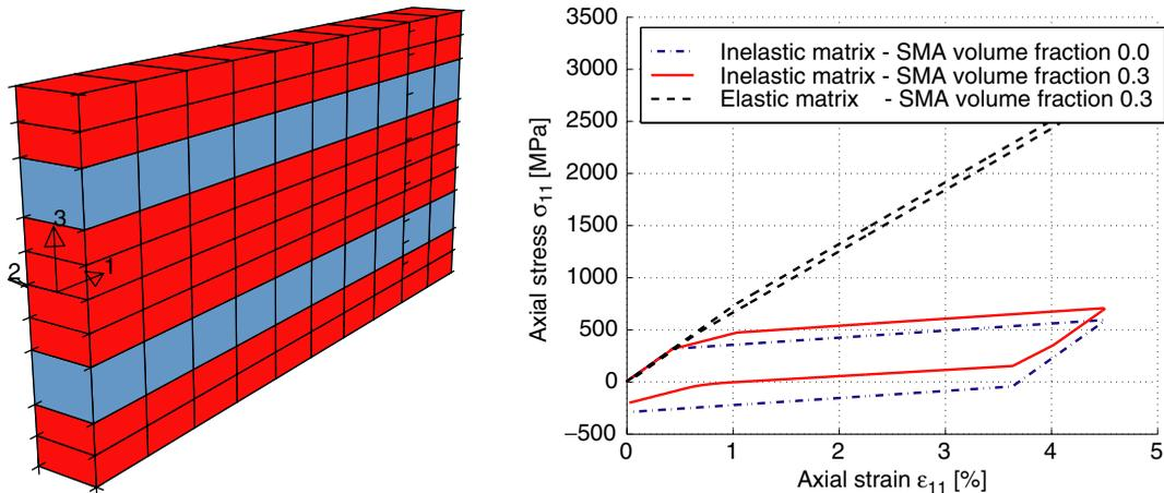
Figure 3. Model of hybrid composite with austenitic SMA wires (volume fraction  $v_w = 0.3$ ) embedded in Aluminium matrix (Problem A) (left part). Axial response comparison between hybrid SMA-Al composite with perfectly elastic matrix, SMA-Al composite with elasto-plastic matrix and Aluminium elasto-plastic matrix without SMA wires (right part).
