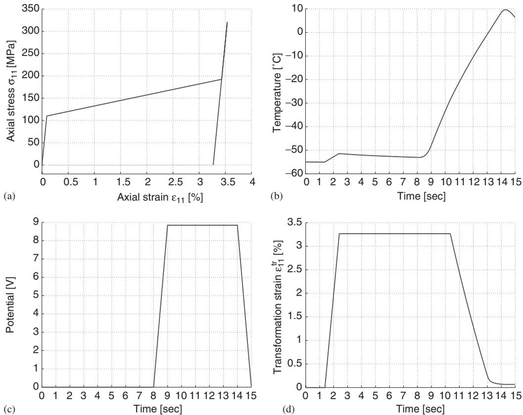
Figure 2. SMA specimen response under mechanical and electrical stimuli. Stress–strain curve during loading–unloading at temperature lower than  $M_f$  (continuous line) and during heating above  $A_f$  (dotted line) (a), temperature (b), potential difference (c) and transformation strain (d) time history.
