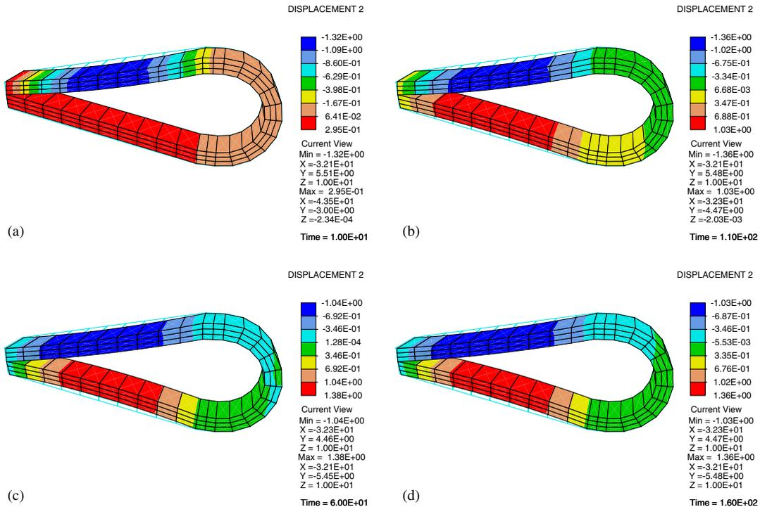
Figure 8. Problem D: vertical displacement changes induced in the composite after the first activation of the upper (a) and the lower (b) SMA wire and after the second activation of the upper (c) and the lower (d) SMA wire.
