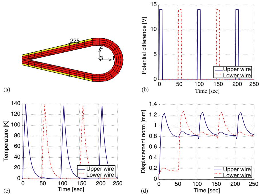
Figure 7. Model of an helicopter blade trailing edge flap (Problem D) (a). Active shape control by SMA wire actuated through Joule effect: potential difference time history of the two highlighted node (b); temperature time history of the two highlighted node (c); freeedge displacement time history of the two highlighted node (d).
