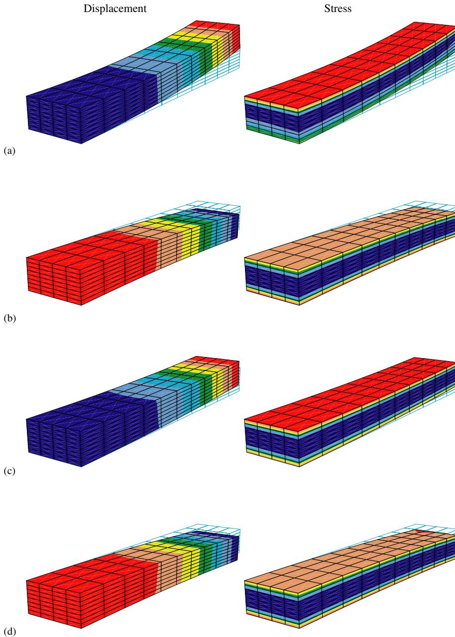
Figure 5. Problem B: vertical displacement (left part) and axial stress (right part) changes induced in the composite after the first activation of the upper (a) and the lower (b) SMA wire and after the second activation of the upper (c) and the lower (d) SMA wire.
