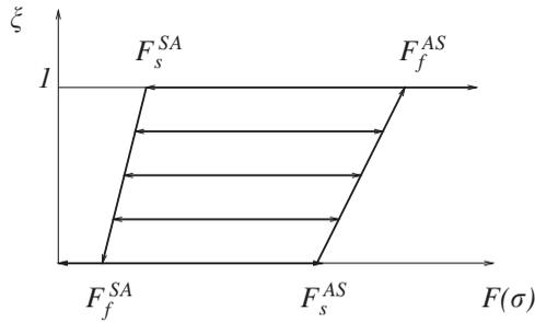
Figure 1. Diagram of relation  $g$ , expressing the dependency of the material fraction  $\zeta$  on the general loading function  $F(\boldsymbol{\sigma})$ . The quantities  $F_s^{AS}$ ,  $F_f^{AS}$ ,  $F_s^{SA}$ ,  $F_f^{SA}$  are material-dependent parameters.
