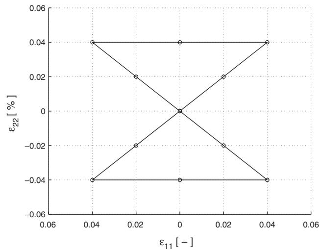
Figure 5. Biaxial test: loading history (in terms of strain  $\varepsilon_{11}$  versus strain  $\varepsilon_{22}$ ) for two different time discretizations.
