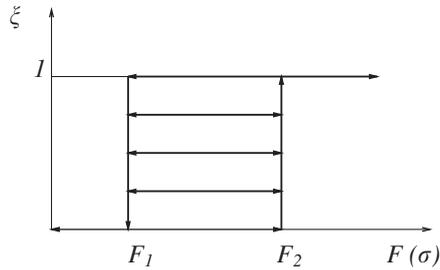
Figure 2. Diagram of relation  $g$ , expressing the dependency of the material fraction  $\zeta$  on the general loading function  $F(\sigma)$ , for the case of no hardening.
