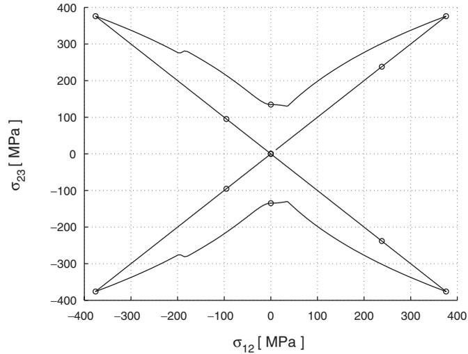
Figure 8. Biaxial torsion test: numerical results (in terms of stress  $\sigma_{12}$  versus stress  $\sigma_{23}$ ) for two different time discretizations.
