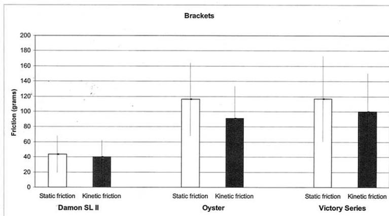
Fig 2. Static and kinetic mean frictions (in grams) and SD of 3 brackets tested.
