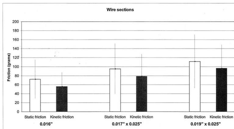
Fig 4. Static and kinetic mean frictions (in grams) and SD of 3 wire sections tested.
