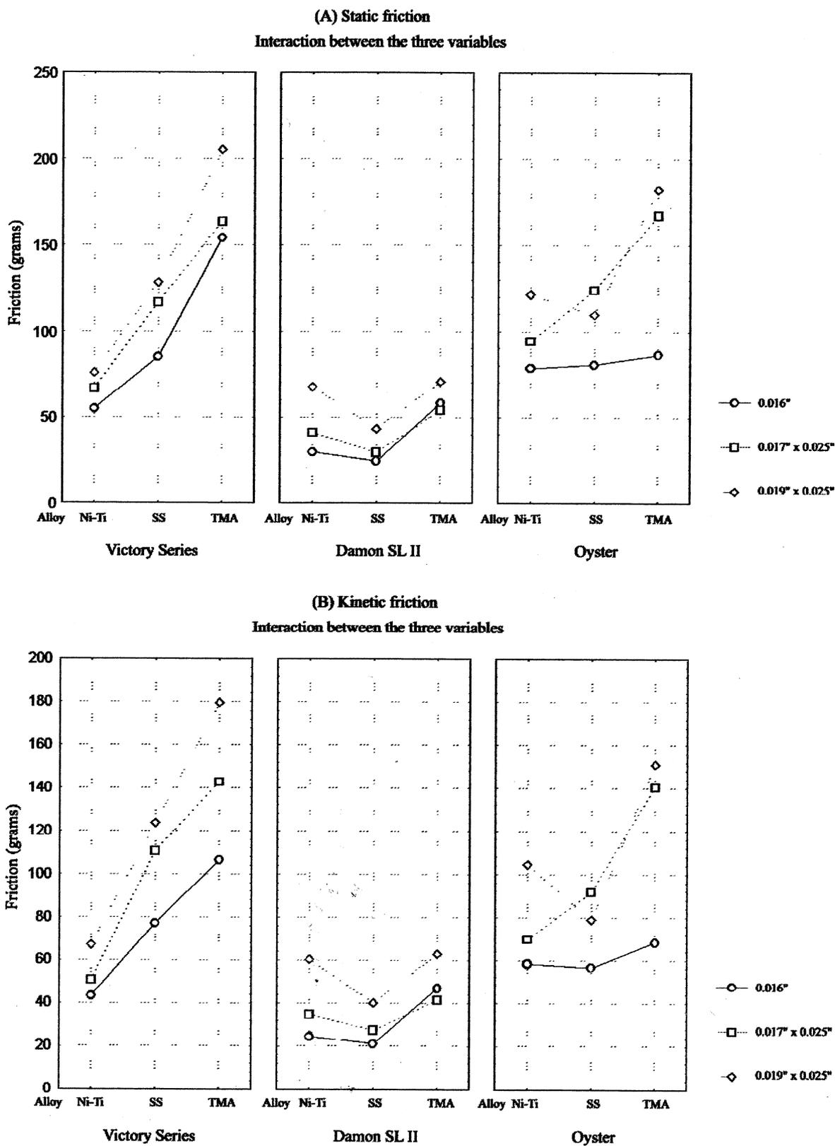
Fig 5. A, Mean static and, B, kinetic friction values of interactions between bracket and alloy for 3 sections investigated.
