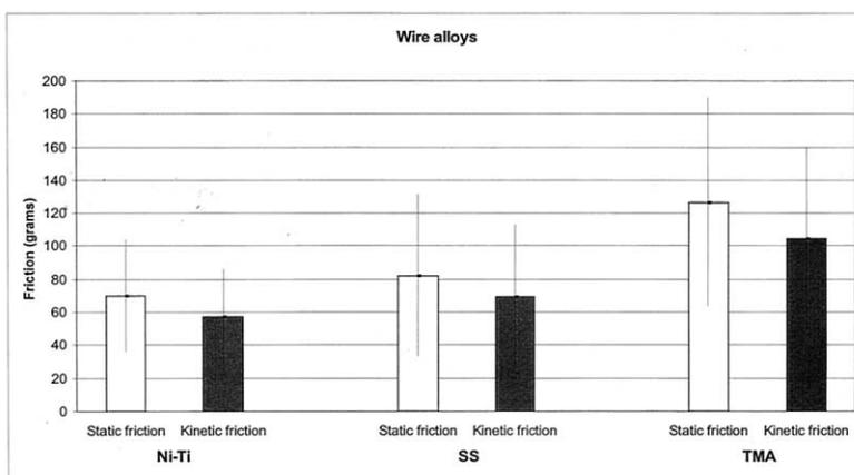
Fig 3. Static and kinetic mean frictions (in grams) and SD of 3 wire alloys tested.
