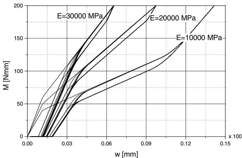
Fig. 9. Bending moment versus transversal displacement for three different values of the Young modulus of the elastic core.
