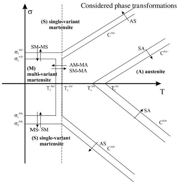
Fig. 1. Scheme of the phase transformation in uniaxial tension and compression versus temperature.
