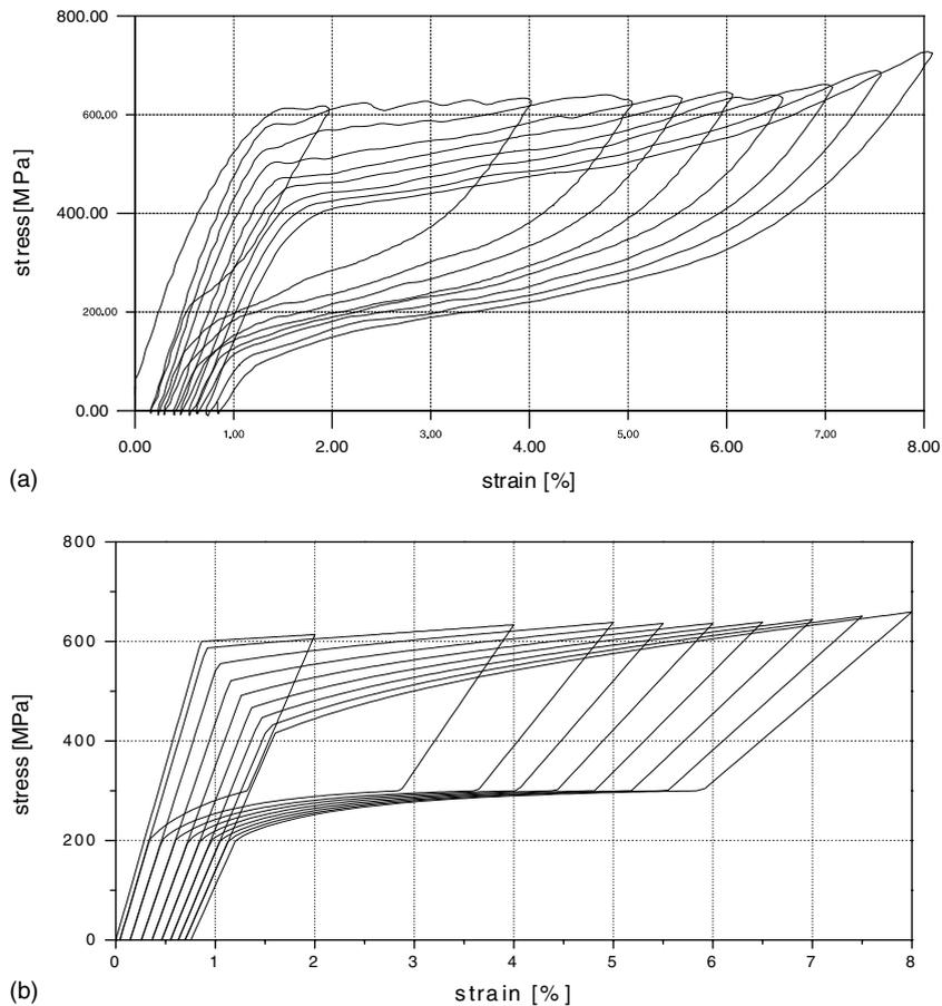
Fig. 6. Pseudoelastic response of a NiTi alloy subjected to loading cycles with an increasing maximum elongation from 2% to 8%: experimental results (a); numerical results (b).
