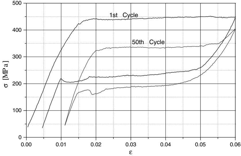
Fig. 2. Stress–strain response of a OMRCO wire of a circular section of Ni–Ti shape memory alloy under cyclic loading: experimental results.
