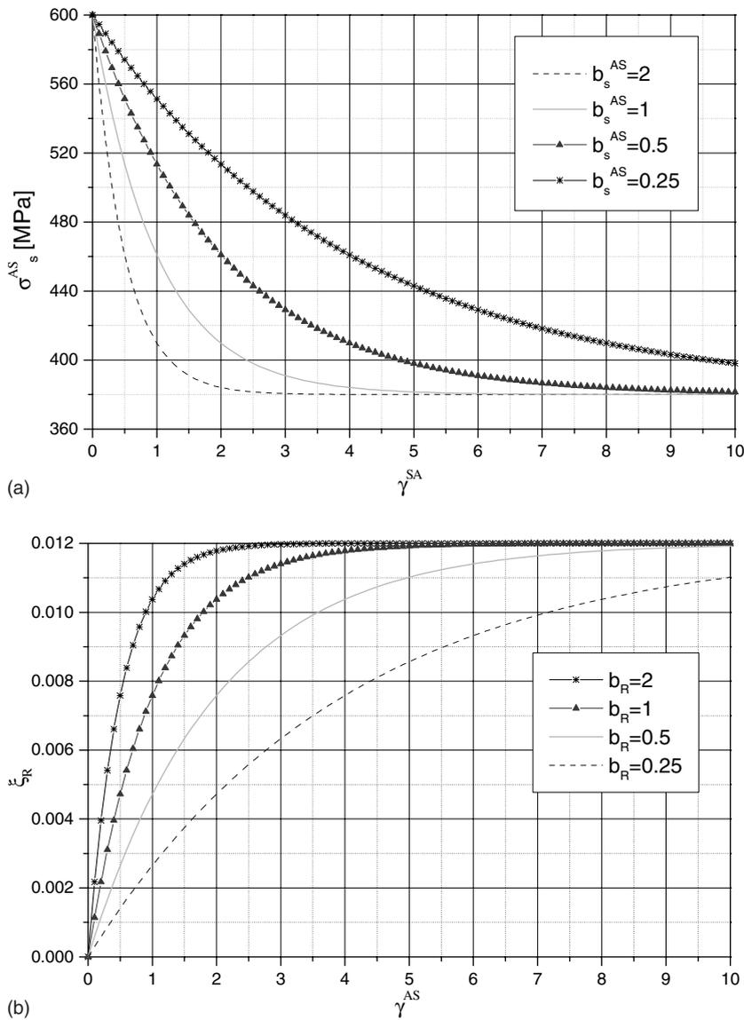
Fig. 3. Evolution  $\sigma_s^{AS}$  of as a function of  $\gamma^{SA}$  for different values of  $b_s^{AS}$  (a); evolution of  $\zeta_R$  as a function of  $\gamma^{AS}$  for different values of  $b_R$  (b).
