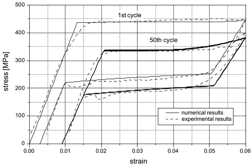
Fig. 8. Stress–strain response of a OMRCO wire under cyclic loading: comparison between experimental and numerical results.
