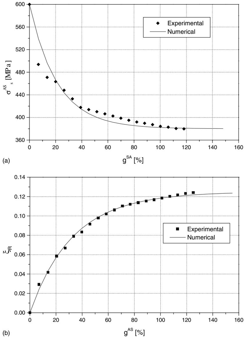
Fig. 5. Evolution of  $\sigma_s^{AS}$  as a function of the accumulated strain  $g^{SA}$  (a); evolution of  $\zeta_R$  as a function of the accumulated strain  $g^{AS}$  (b).
