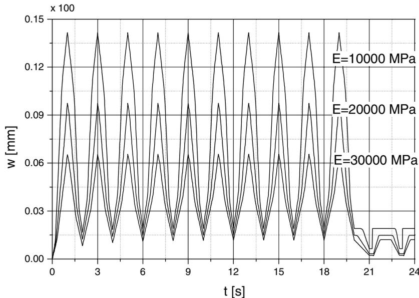
Fig. 10. Transversal displacement versus time for three different values of the Young modulus of the elastic core.
