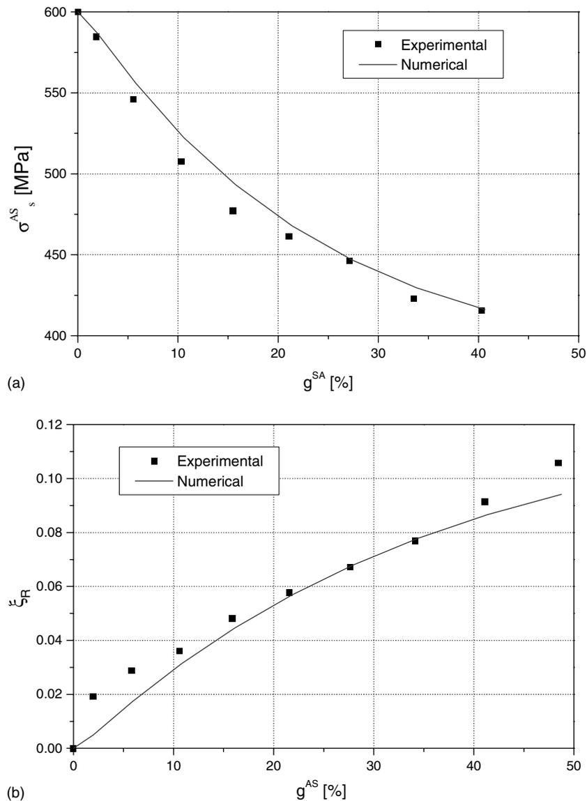
Fig. 7. Evolution of  $\sigma_s^{AS}$  as a function of the accumulated strain  $g^{SA}$  (a); evolution of  $\zeta_R$  as a function of the accumulated strain  $g^{AS}$  (b).
