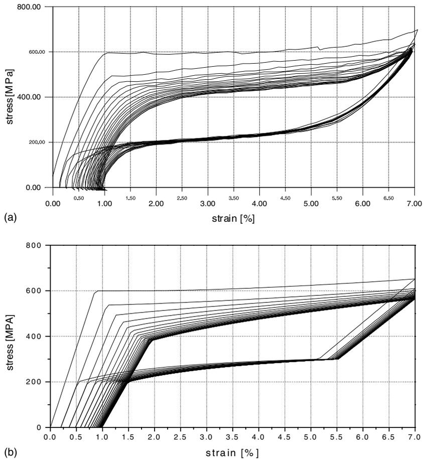
Fig. 4. Pseudoelastic response of a NiTi alloy subjected to equal loading cycles with 7% maximum elongation: experimental results (a); numerical results (b).
