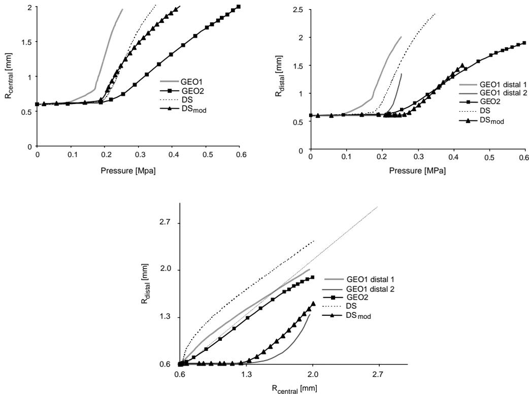
Fig. 6. Comparison of the central and distal radius expansion at different values of internal pressure (top) and comparison between distal and central radius (bottom) for models DS, DS<sub>mod</sub>, GEO1 and GEO2; dot lines as in Fig. 4.
