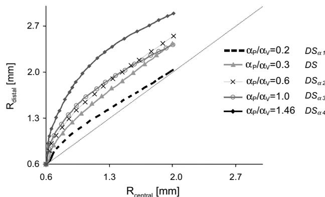
Fig. 4. Expansion of the distal and central radius for the DS stents: reducing the metal-to-artery ratio and increasing the inflation pressure, the expansion tends to become uniform along the stent; dot lines represent the uniform stent expansion.
