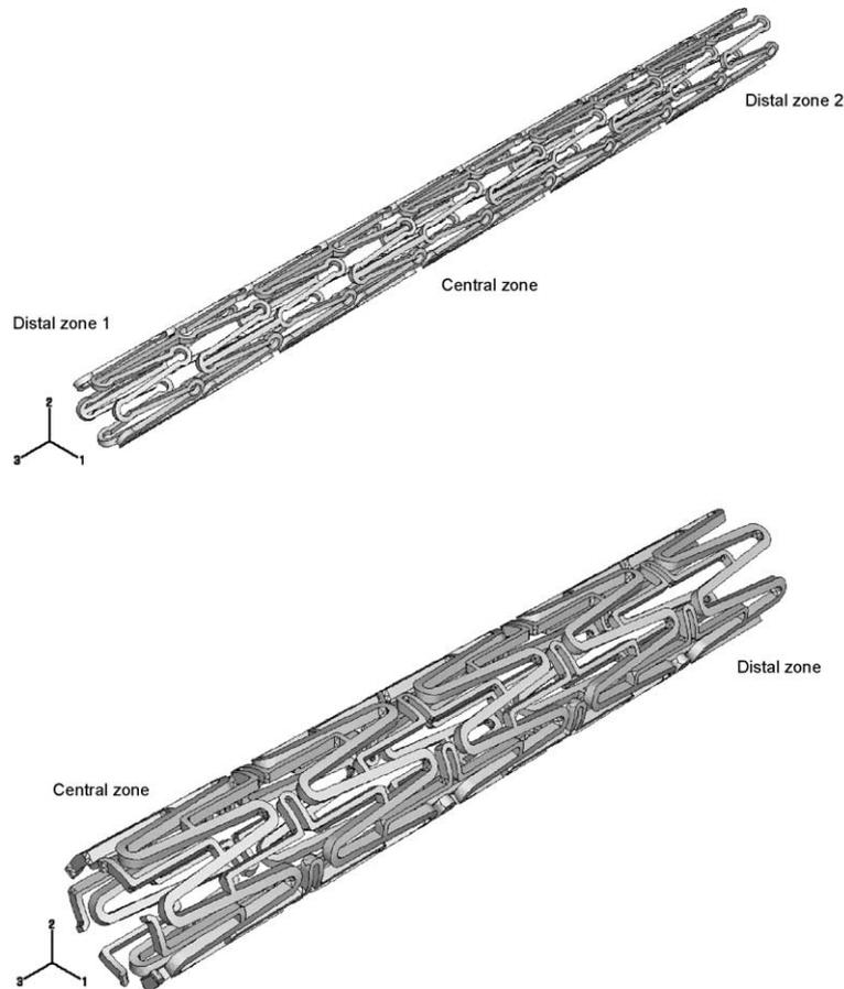
Fig. 2. GEO1 (top) and GEO2 (bottom) models. The former is complete, as there are no geometrical symmetries, while the latter is represented only for a half of its length.
