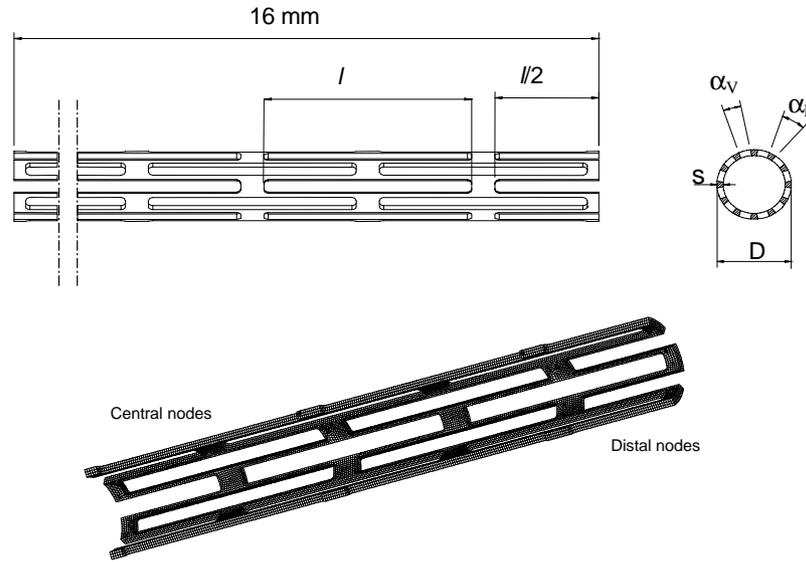
Fig. 1. Geometry of the unexpanded DS stent strut;  $l$ : length of the slot,  $s$ : thickness,  $\alpha_p$ : angle described by the metallic surface,  $\alpha_v$ : angle described by the slot and  $D$ : outer diameter; finite element mesh for a quarter of model DS stent.
