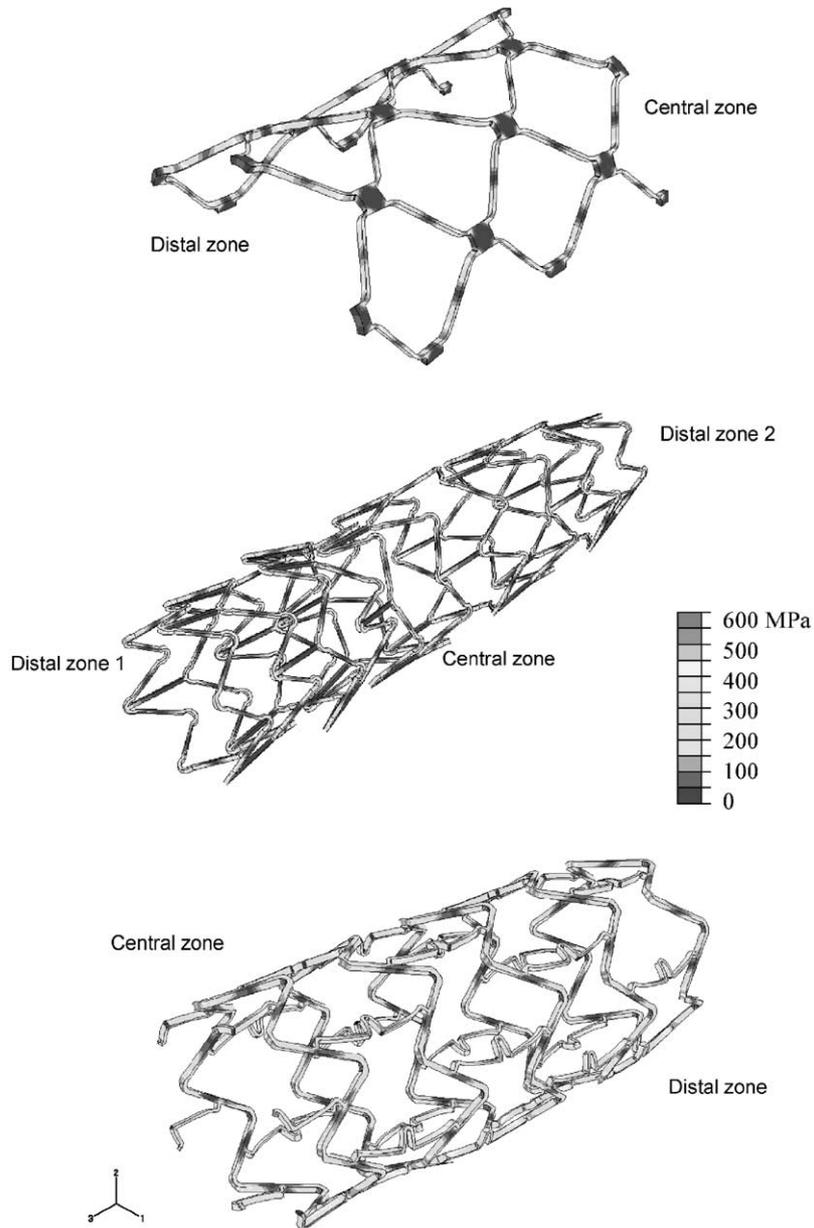
Fig. 5. Von Mises stress contours for models DS, GEO1 and GEO2<sup>4</sup>.
