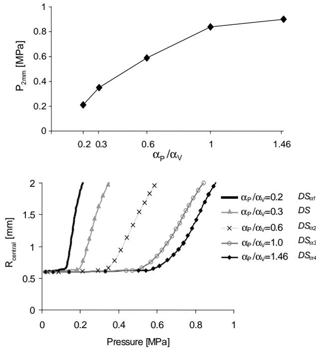
Fig. 3. Top: pressure necessary ( $P_{2\text{mm}}$ ) to reach a radius equal to 2 mm in the central zone as a function of the metal-to-artery ratio; bottom: central radius as function of the pressure for models with different metal-to-artery ratio.
