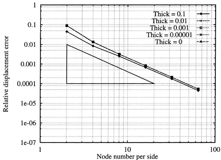
Fig. 6. Q4-LIM element. Relative deflection error versus number of nodes per side for different values of thickness. It can be observed the attainment of the  $h^2$  convergence rate in the  $L^2$  error norm, corresponding to a  $h$  convergence rate in the  $H^1$  energy-type norm.
