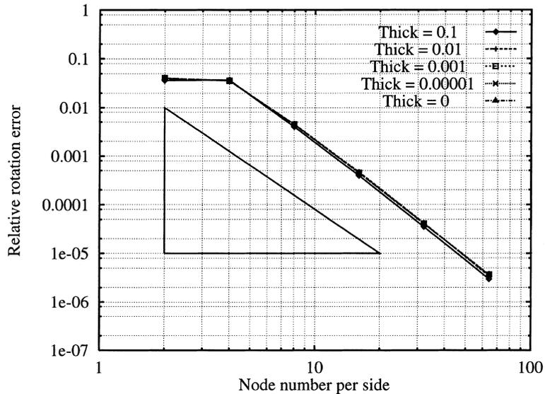
Fig. 3. T9-LIM element. Relative rotation error versus number of nodes per side for different values of thickness. It can be observed the attainment of the  $h^3$  convergence rate in the  $L^2$  error norm, corresponding to a  $h^2$  convergence rate in the  $H^1$  energy-type norm.
