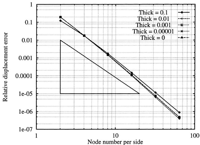
Fig. 4. T9-LIM element. Relative deflection error versus number of nodes per side for different values of thickness. It can be observed the attainment of the  $h^3$  convergence rate in the  $L^2$  error norm, corresponding to a  $h^2$  convergence rate in the  $H^1$  energy-type norm.
