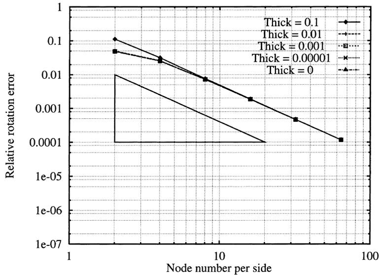
Fig. 5. Q4-LIM element. Relative rotation error versus number of nodes per side for different values of thickness. It can be observed the attainment of the  $h^2$  convergence rate in the  $L^2$  error norm, corresponding to a  $h$  convergence rate in the  $H^1$  energy-type norm.
