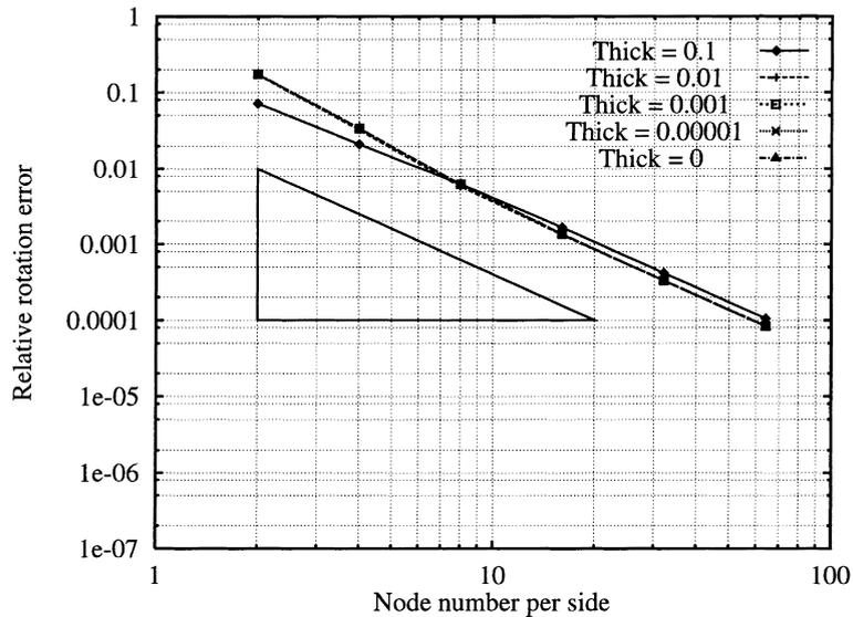
Fig. 1. T3-LIM element. Relative rotation error versus number of nodes per side for different values of thickness. It can be observed the attainment of the  $h^2$  convergence rate in the  $L^2$  error norm, corresponding to a  $h$  convergence rate in the  $H^1$  energy-type norm.
