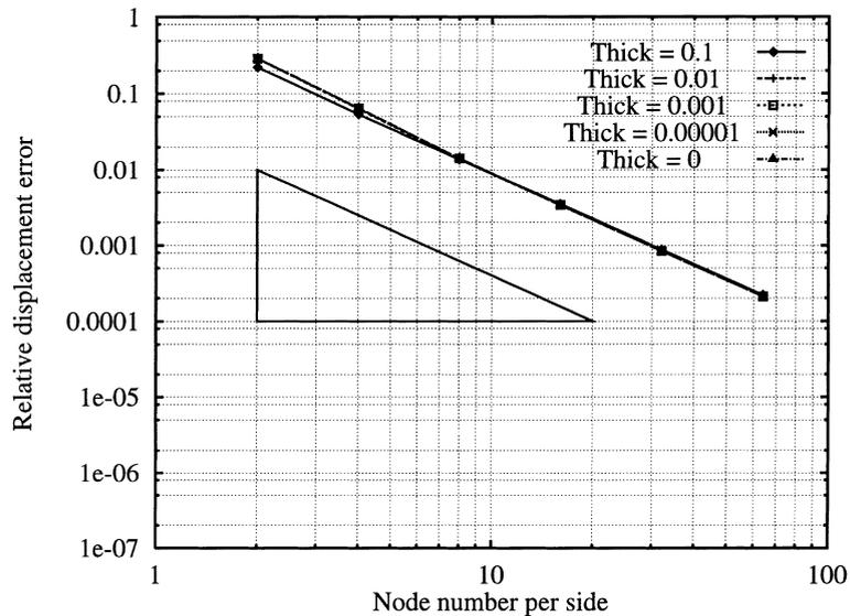
Fig. 2. T3-LIM element. Relative deflection error versus number of nodes per side for different values of thickness. It can be observed the attainment of the  $h^2$  convergence rate in the  $L^2$  error norm, corresponding to a  $h$  convergence rate in the  $H^1$  energy-type norm.
