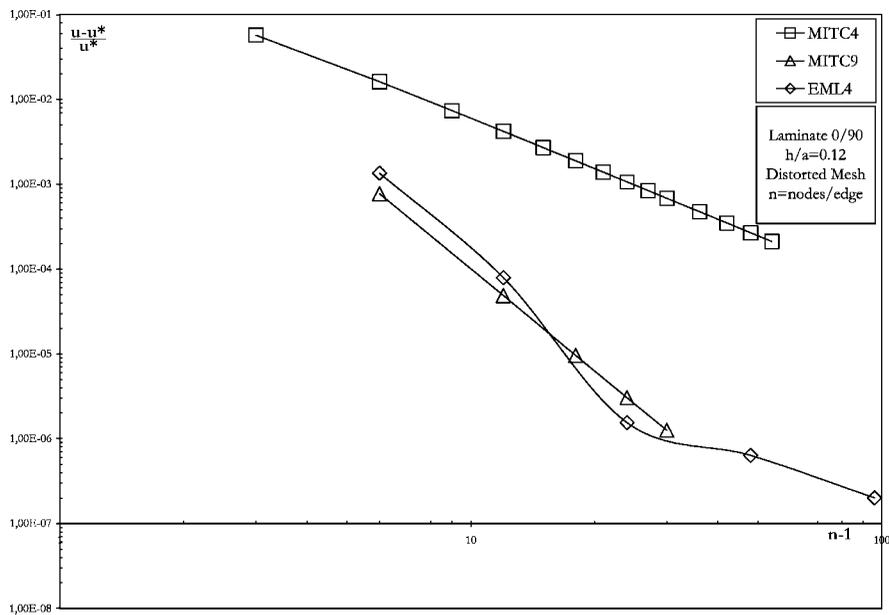
Figure 3. Convergence analysis for mid-plate vertical displacement (Point A)—distorted mesh.
