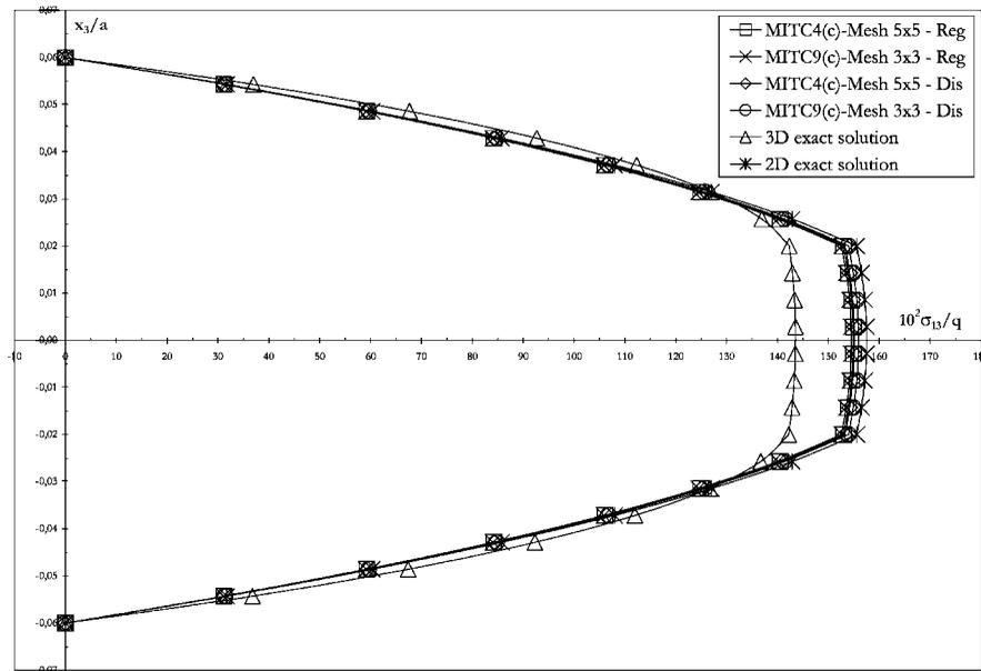
Figure 9. Through-the-thickness distributions of stress  $\sigma_{13}$  at  $x = y = a/4$ ; Laminate 0/90/0.
