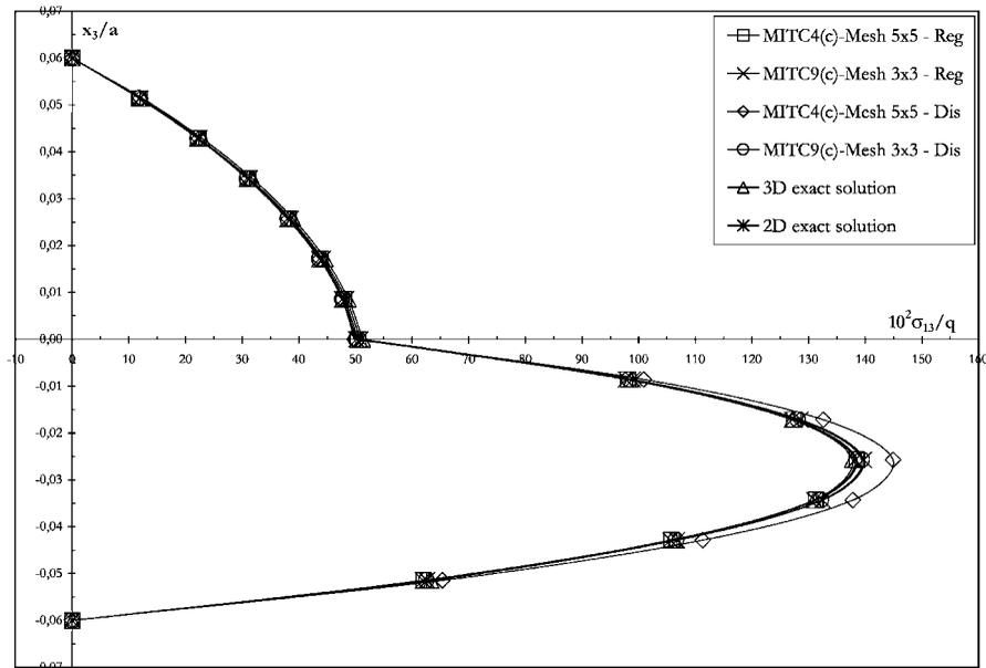
Figure 8. Through-the-thickness distributions of stress  $\sigma_{13}$  at  $x = y = a/4$ ; Laminate 0/90.
