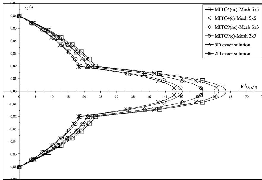
Figure 18. Through-the-thickness distributions of corrected (c) and non-corrected (nc) stress  $\sigma_{23}$  at  $x = y = a/4$ ; Laminate 0/90/0, distorted mesh.
