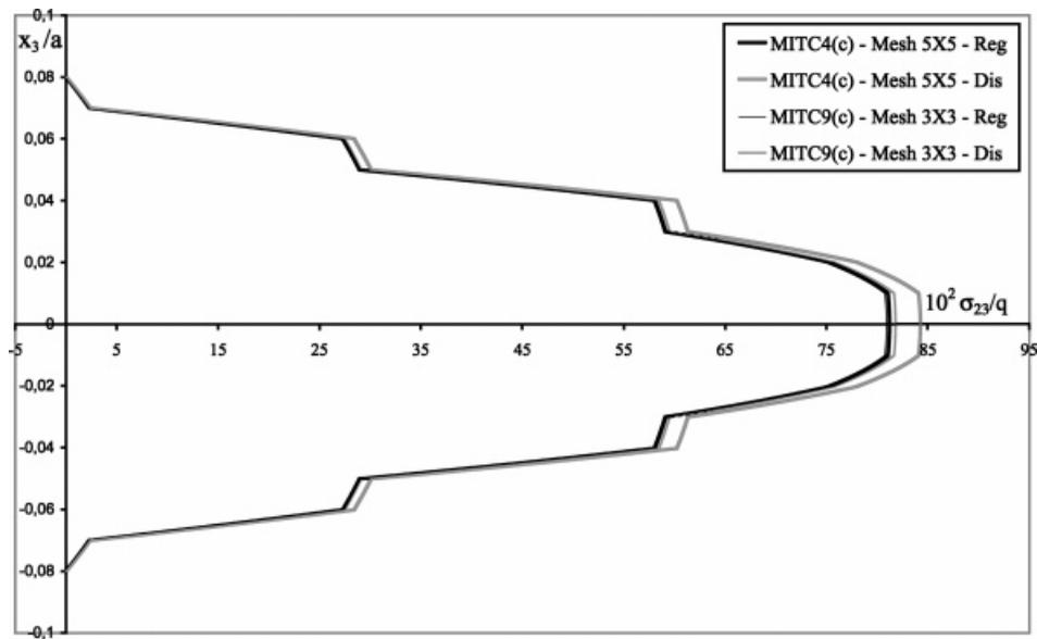
Figure 24. Through-the-thickness distributions of corrected (c) stress  $\sigma_{23}$  at  $x = y = a/4$  for regular (Reg) and distorted (Dis) meshes; Laminate  $(0/90/-45/45/-45/45/90/0)_{\text{sym}}$ .
