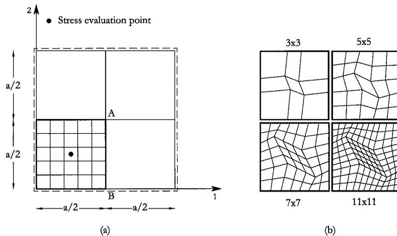
Figure 1. Simply supported plate: finite element meshes and geometric data:
