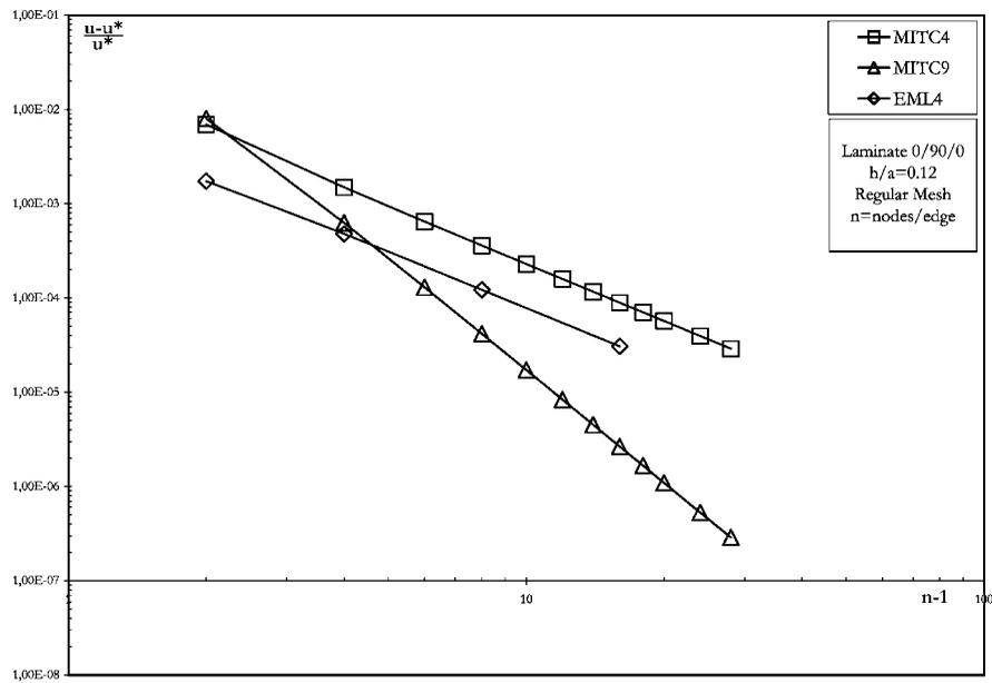
Figure 6. Convergence analysis for mid-plate vertical displacement (Point A)—regular mesh.
