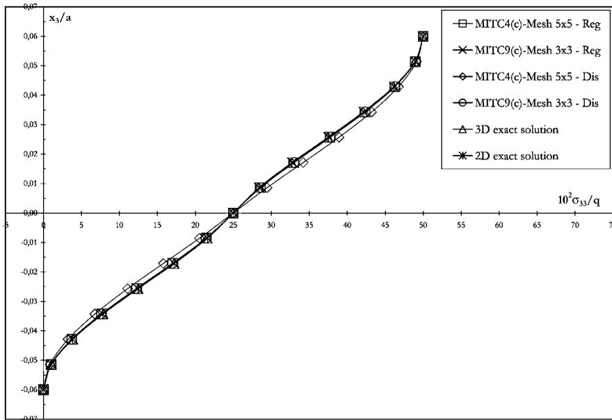
Figure 11. Through-the-thickness distributions of stress  $\sigma_{33}$  at  $x = y = a/4$ ; Laminate 0/90.
