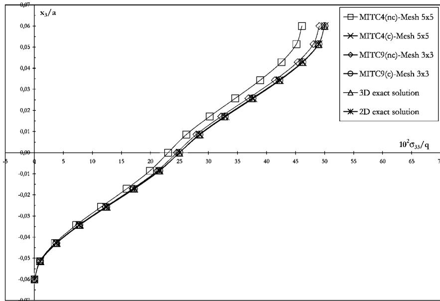
Figure 19. Through-the-thickness distributions of corrected (c) and non-corrected (nc) stress  $\sigma_{33}$  at  $x = y = a/4$ ; Laminate 0/90, regular mesh.
