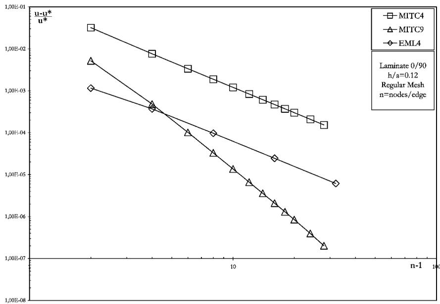
Figure 2. Convergence analysis for mid-plate vertical displacement (Point A)—regular mesh.
