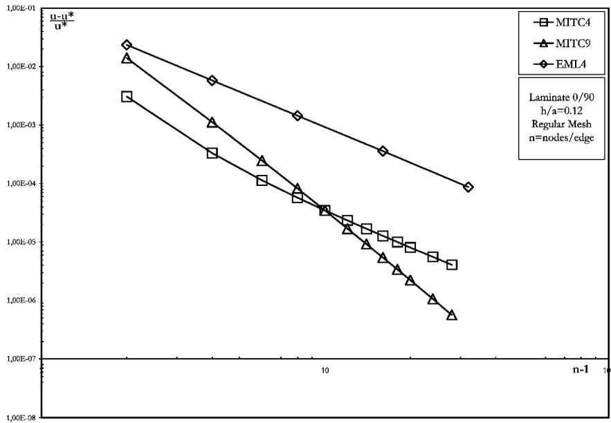
Figure 4. Convergence analysis for mid-side horizontal displacement (Point B)—regular mesh.
