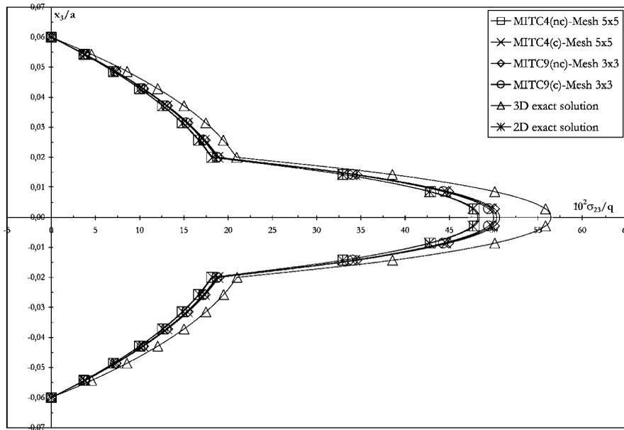
Figure 17. Through-the-thickness distributions of corrected (c) and non-corrected (nc) stress  $\sigma_{23}$  at  $x = y = a/4$ ; Laminate 0/90/0, regular mesh.
