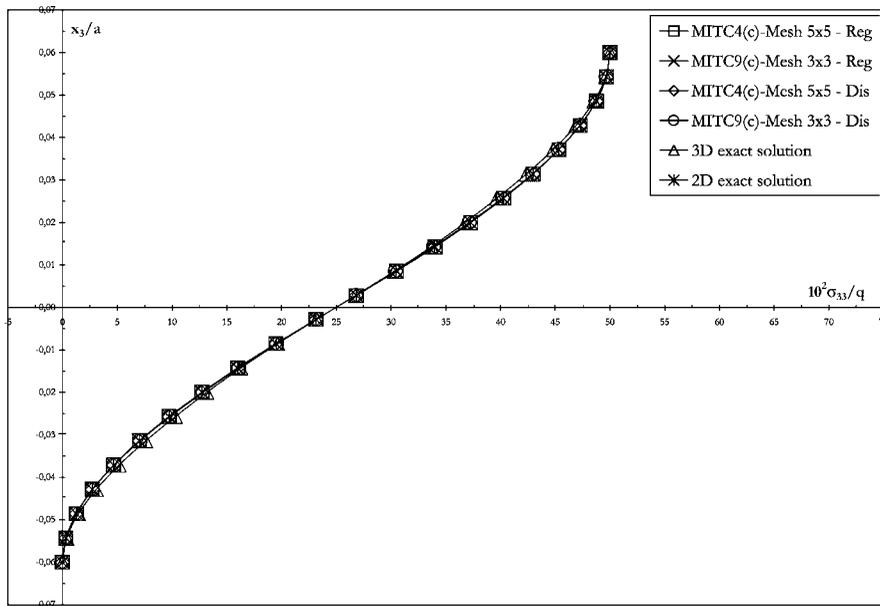
Figure 12. Through-the-thickness distributions of stress  $\sigma_{33}$  at  $x = y = a/4$ ; Laminate 0/90/0.
