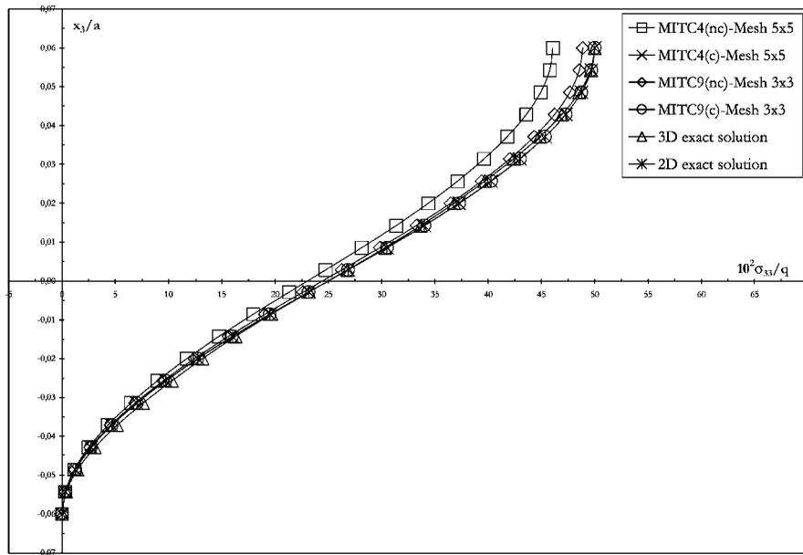
Figure 21. Through-the-thickness distributions of corrected (c) and non-corrected (nc) stress  $\sigma_{33}$  at  $x = y = a/4$ ; Laminate 0/90/0, regular mesh.
