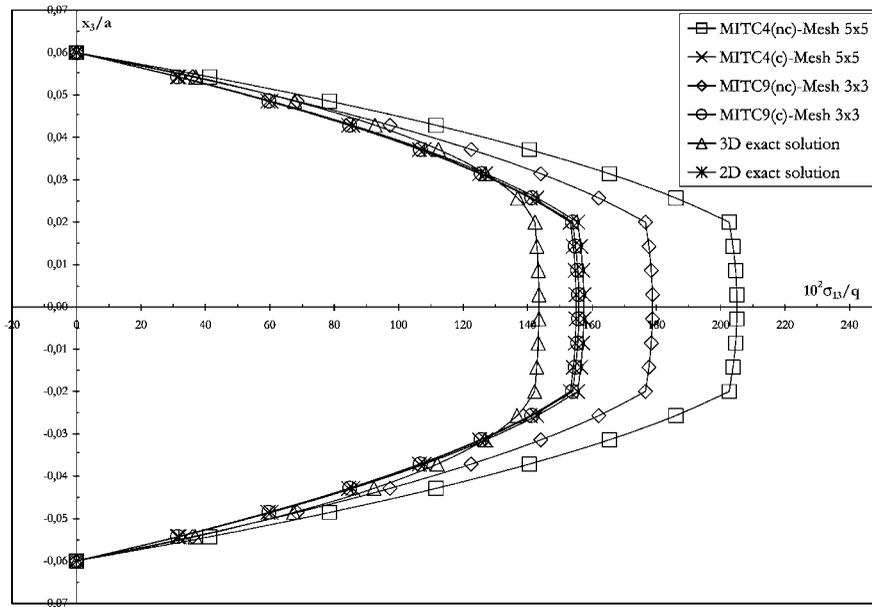
Figure 16. Through-the-thickness distributions of corrected (c) and non-corrected (nc) stress  $\sigma_{13}$  at  $x = y = a/4$ ; Laminate 0/90/0, distorted mesh.
