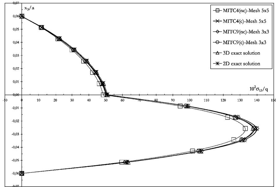
Figure 13. Through-the-thickness distributions of corrected (c) and non-corrected (nc) stress  $\sigma_{13}$  at  $x = y = a/4$ ; Laminate 0/90, regular mesh.
