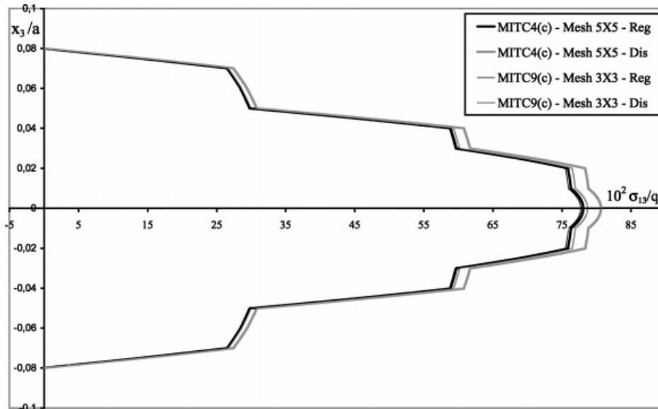
Figure 23. Through-the-thickness distributions of corrected (c) stress  $\sigma_{13}$  at  $x = y = a/4$  for regular (Reg) and distorted (Dis) meshes; Laminate  $(0/90/-45/45/-45/45/90/0)_{\text{sym}}$ .
