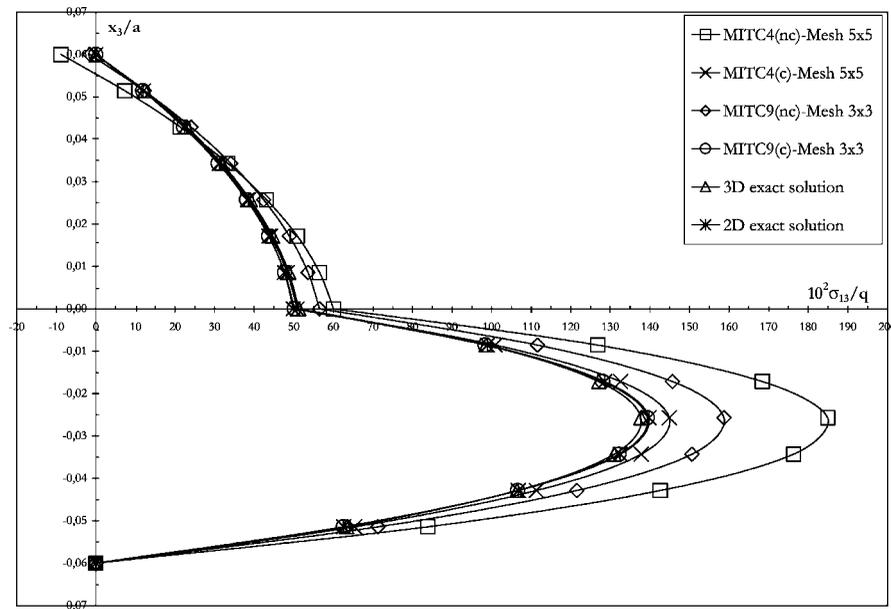
Figure 14. Through-the-thickness distributions of corrected (c) and non-corrected (nc) stress  $\sigma_{13}$  at  $x = y = a/4$ ; Laminate 0/90, distorted mesh.
