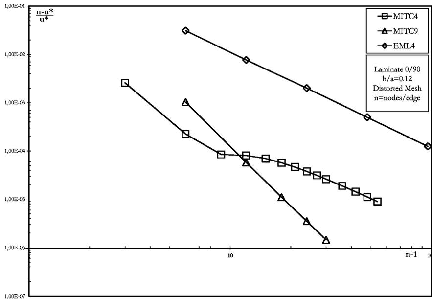
Figure 5. Convergence analysis for mid-side horizontal displacement (Point B)—distorted mesh.
