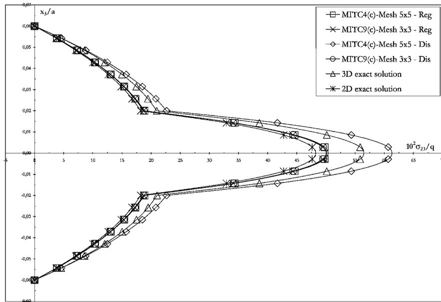
Figure 10. Through-the-thickness distributions of stress  $\sigma_{23}$  at  $x = y = a/4$ ; Laminate 0/90/0.
