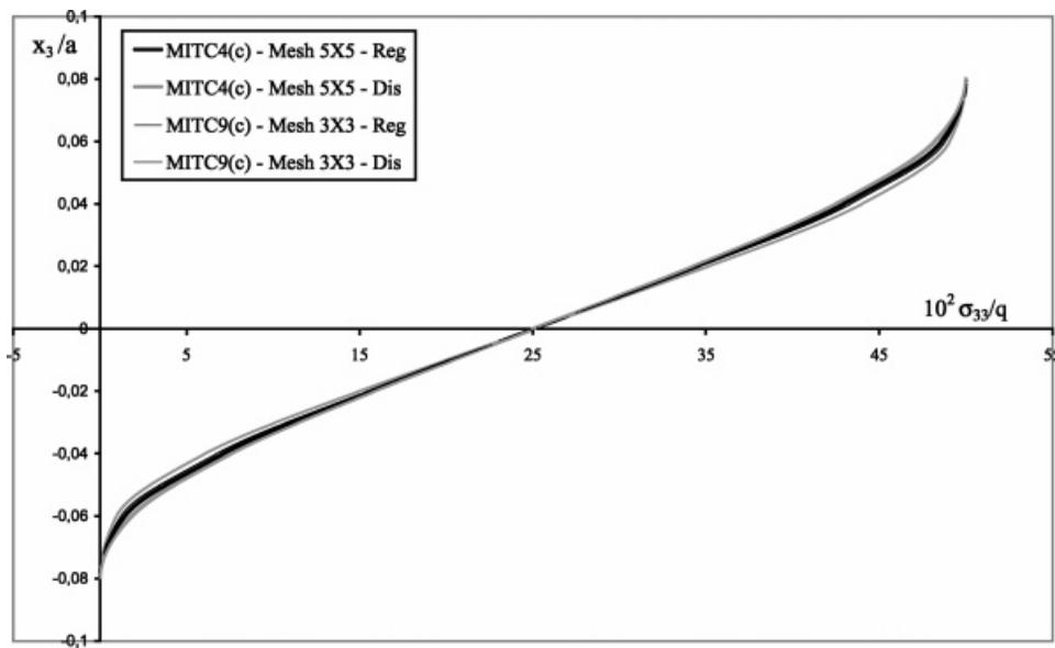
Figure 25. Through-the-thickness distributions of corrected (c) stress  $\sigma_{33}$  at  $x = y = a/4$  for regular (Reg) and distorted (Dis) meshes; Laminate  $(0/90/-45/45/-45/45/90/0)_{\text{sym}}$ .
