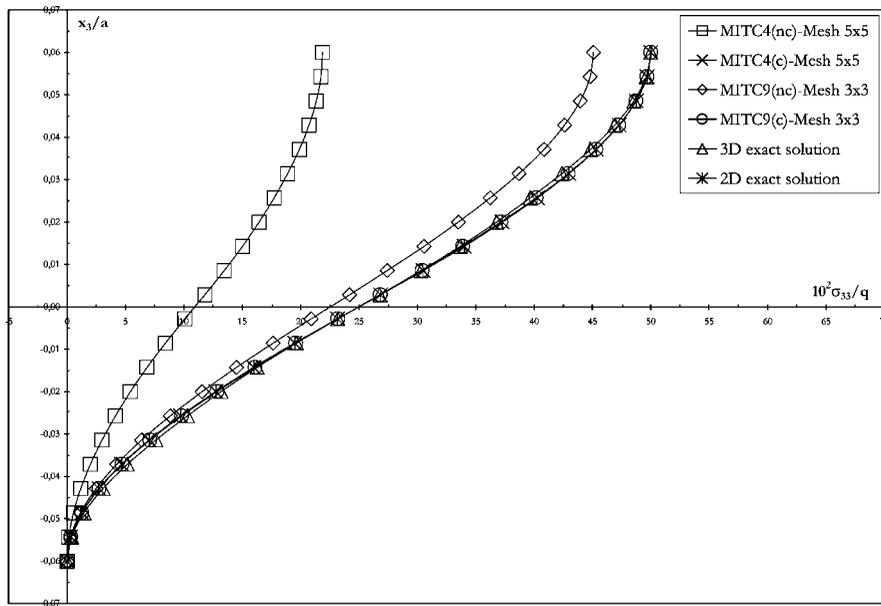
Figure 22. Through-the-thickness distributions of corrected (c) and non-corrected (nc) stress  $\sigma_{33}$  at  $x = y = a/4$ ; Laminate 0/90/0, distorted mesh.
