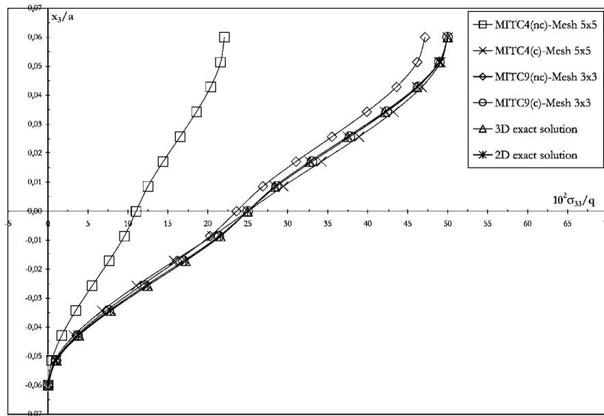
Figure 20. Through-the-thickness distributions of corrected (c) and non-corrected (nc) stress  $\sigma_{33}$  at  $x = y = a/4$ ; Laminate 0/90, distorted mesh.
