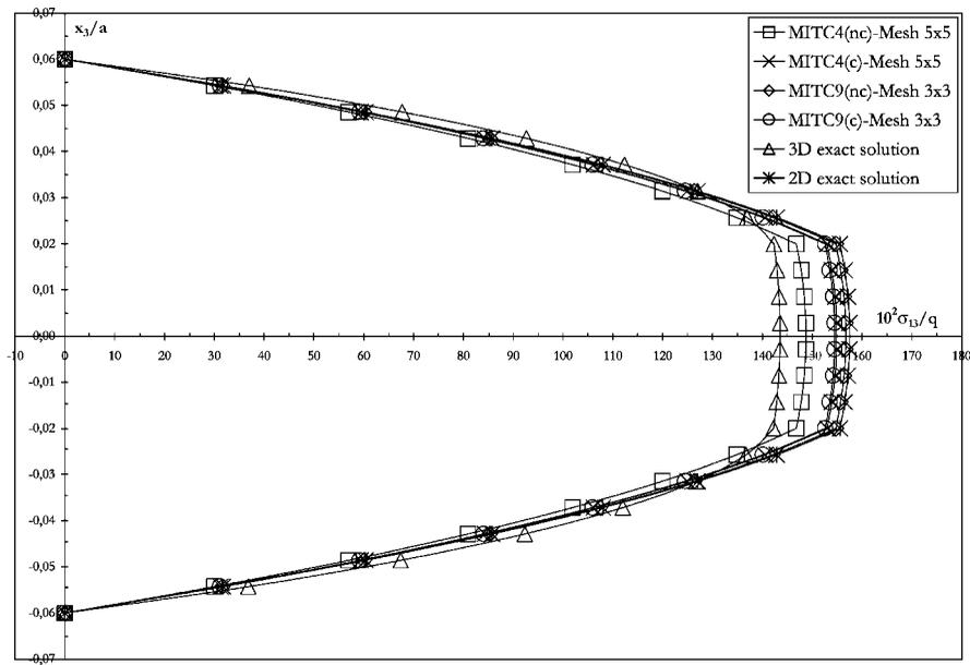
Figure 15. Through-the-thickness distributions of corrected (c) and non-corrected (nc) stress  $\sigma_{13}$  at  $x = y = a/4$ ; Laminate 0/90/0, regular mesh.
