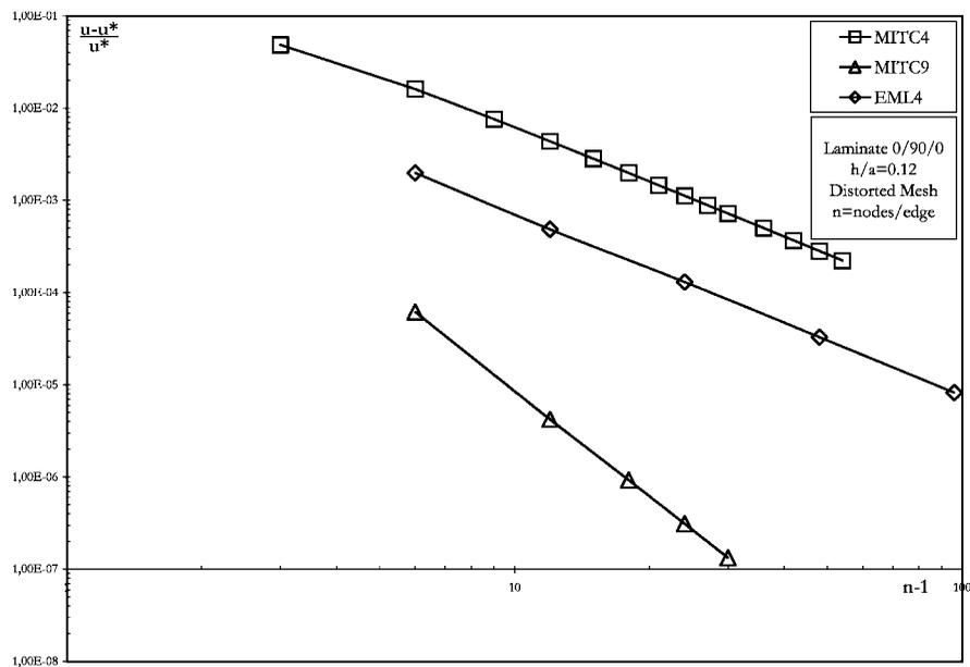
Figure 7. Convergence analysis for mid-plate vertical displacement (Point A)—distorted mesh.
