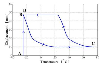
Spring actuator. Vertical displacement of the lower loaded end of spring versus temperature variation.
