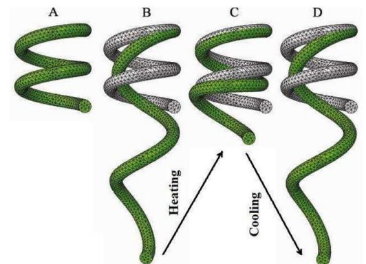
Spring actuator. A) initial geometry; B) deformed shape due to the weight application at  $T = -25^\circ\text{C}$ ; C) spring shape recovery and weight lifting due to heating to  $T = 100^\circ\text{C}$ ; D) spring stretching due to cooling to  $T = -25^\circ\text{C}$ .
