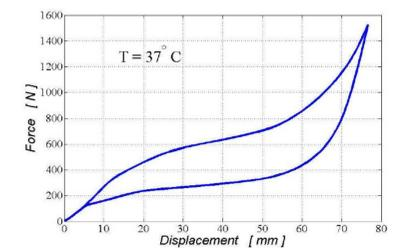
Pseudo-elasticity. Force-displacement diagram for SMA spring.
