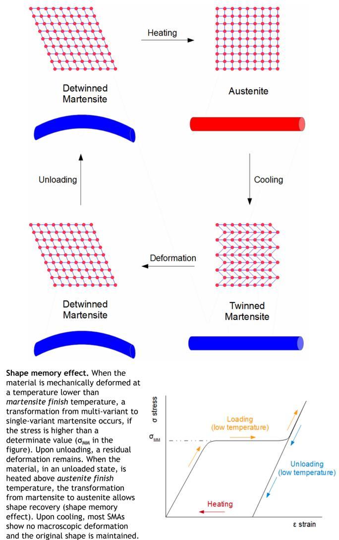
SMA particular characteristics allow a variety of innovative applications in different engineering fields, such as biomedical (e.g. stents, surgery tools, active implants), structural (e.g. damping devices), automotive (e.g. actuators), aeronautical (e.g. the Variable Geometry Chevron), mechanical (e.g. heat engines, coupling devices) and robotic (e.g. SMA actuated microrobots) engineering.
