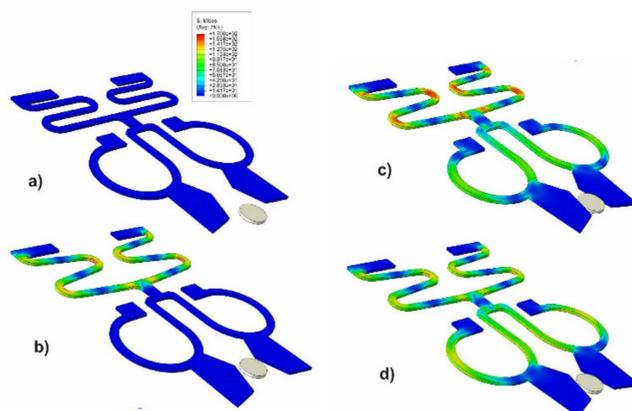
Simulation of micro-gripper with a sample. a) starting configuration; b) memorization step; c) heating of linear actuator and sample gripping; d) heating of rotary actuator with consequent re-opening. von Mises stress [MPa] distribution in the micro-gripper are depicted in the contour plot.
