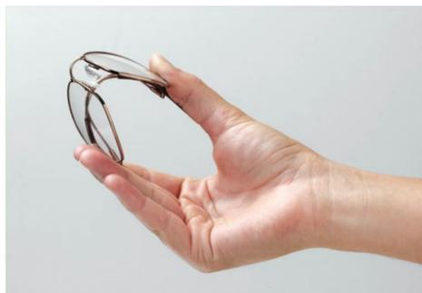
Shape memory eyeglass frame. Shape memory eyeglass frame is a real life example of superelastic behavior. It can undergo severe deformation and still recover original shape.
